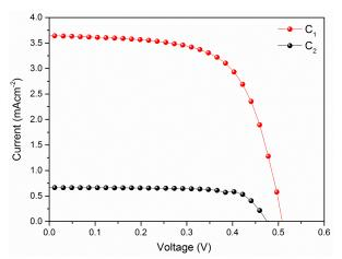
Fig. 6 – J-V characteristics of DSSCs sensitized with dyes  $\mathbf{C}_1$  and  $\mathbf{C}_2$
