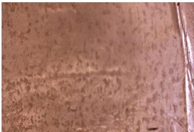
Fig. 4 – Deposition of copper ions on AFS at the 12 V and 18 g/l concentrated electrolyte solution.
