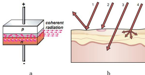
**Fig. 1** – Structure of a diode laser (a); processes in biological tissue under the influence of laser radiation (b): 1 – reflection; 2 – absorption; 3 – transmission, 4 – scatter
