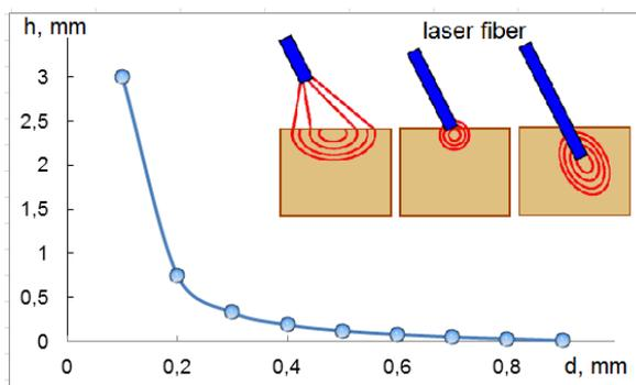
Fig. 3 – Experimental dependence of the cutting depths versus the diameter of the laser beam at a wavelength  $\lambda = 980$  nm and time of laser exposure  $\tau = 5$  s
