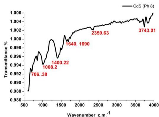
Fig. 6 – FTIR spectrum of CdS I sample
