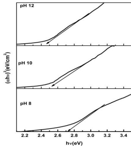
Fig. 3 – Tauc plot of CdS nanoparticles with different pH
