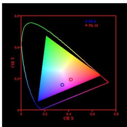
Fig. 5 – CIE plot of CdS nanoparticles
