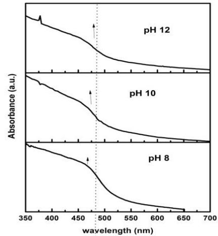
Fig. 2 – UV-Vis absorption spectra of CdS nanoparticles with different pH value
