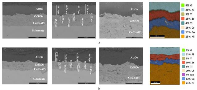
**Fig. 2** – SEM micrographs of cross-sections of the CoCrAlY/ZrSiO<sub>4</sub>/Al<sub>2</sub>O<sub>3</sub> coatings (back-scattered electron mode, Quanta 200 3D) before (a) and after (b) thermal treatment and SEM EDX element distribution maps (NanoSEM 450)
