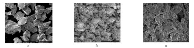
Fig. 1 – Morphology of the CoCrAlY (a), ZrSiO<sub>4</sub> (b), and Al<sub>2</sub>O<sub>3</sub> (c) powders (SEM)
