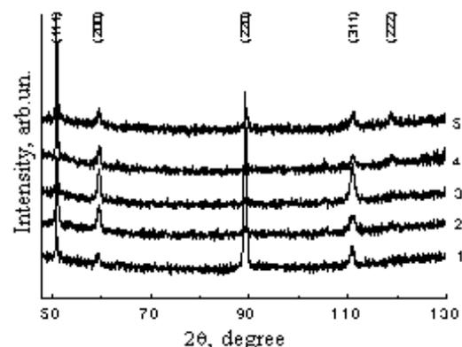
Fig. 2 – The diffraction patterns obtained from the BL1-BL5 fragments (the number near the diffraction pattern corresponds to the fragment number)
