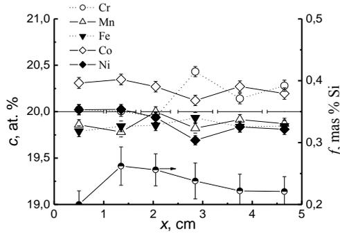
**Fig. 5** – Distribution of element concentration (at. %) over the length of the sample obtained from the average concentration of elements of BL1-BL5 fragments (right axis – concentration (at. %) of impurity silicon along the length)
