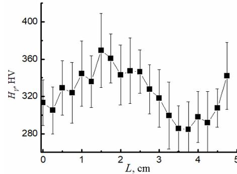
Fig. 1 – The distribution of microhardness, HV, along the length  $L$  of the sample of the FeCrMnCoNi HEA
