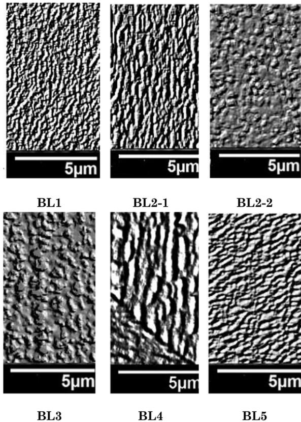
**Fig. 4** – SEM images of the surface of the fragments BL1-BL5
