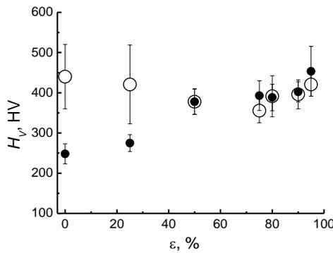
**Fig. 7** – Dependence of microhardness,  $H_V$ , on the magnitude of rolling deformation,  $\varepsilon$ , of samples deformed without annealing (light circles) and annealed at 950 °C for 30 min before rolling (dark circles)
