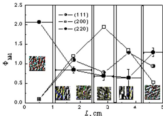
**Fig. 3** –  $\Phi_{hkl}$  parameters of Wilson calculated from the intensities of the (111), (200) and (220) diffraction maxima for the BL1-BL5 fragments. The length of each fragment is limited by parallel lines, the distance between which corresponds to the part of the sample removed from the sample when cut into fragments. On the insets: the microstructure of the central part of each fragment
