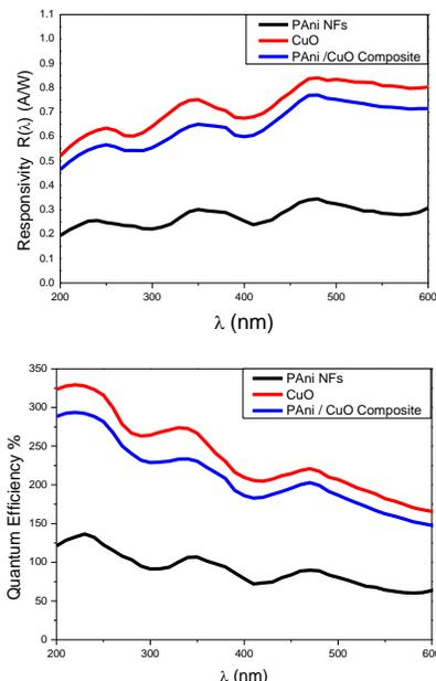
Fig 5 – The variation of spectral responsivity and QE with wavelength for PAni NFs, CuO and PAni/CuO composite
