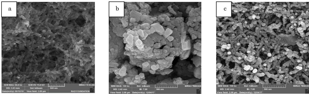
Fig. 2 – SEM images of PANi NFs (a), CuO (b) and PANi/CuO nanocomposite (c)
