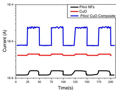
Fig 4 – Photoresponse time of samples as UV photodetector upon exposure to 250 nm
