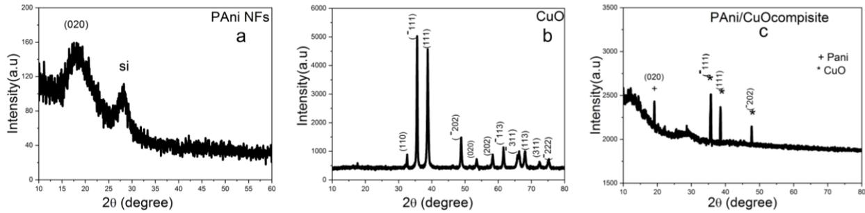
Fig. 1 – X-ray of PANi NFs (a), CuO thin film (b) and PANi/CuO composite (c)
