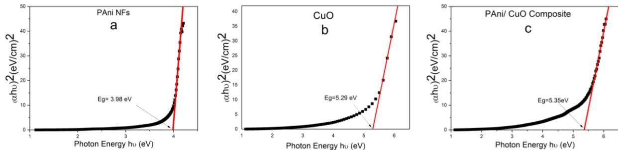
Fig. 3 – Energy gap for PANi NFs (a), CuO nanostructures (b) and PANi/CuO composite (c)
