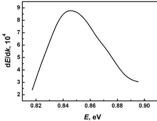
Fig. 3 – Determination of the band gap width at the maximum of the differentiated absorption curve
