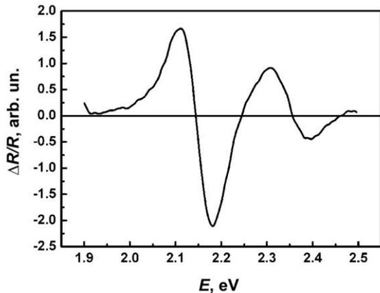
Fig. 6 – Electroreflectance spectra of the germanium films (region of  $E_1$  and  $E_1 + \Delta_1$  transitions)
