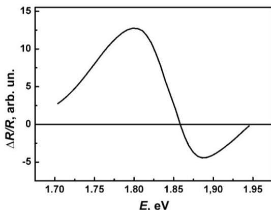
Fig. 8 – Electroreflectance spectra of the gallium arsenide substrate (region of  $E_0 + \Delta_0$  transitions)
