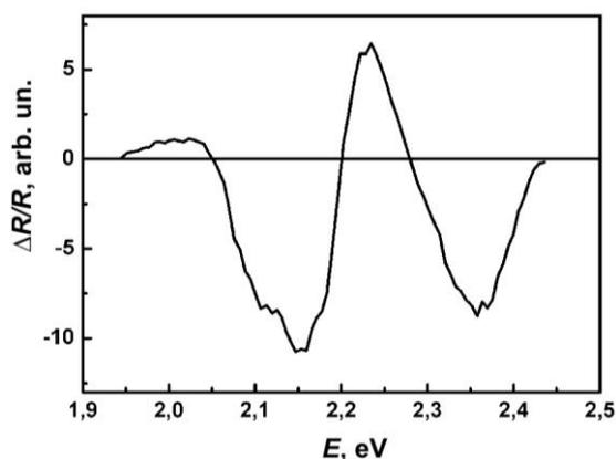
Fig. 7 – Electroreflectance spectra of the germanium with gallium films (region of  $E_1$  and  $E_1 + \Delta_1$  transitions)
