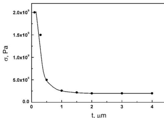
Fig. 1 – Dependence of the internal mechanical compressive stresses in Ge films on GaAs on the film thickness. The deposition temperature was 300  $^{\circ}\text{C}$
