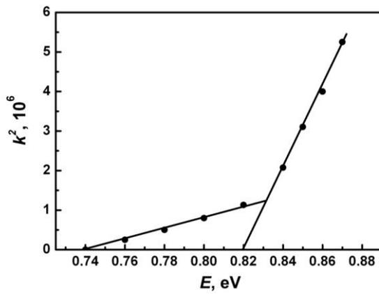
Fig. 4 – Spectral dependence of  $k^2$  for germanium with gallium film
