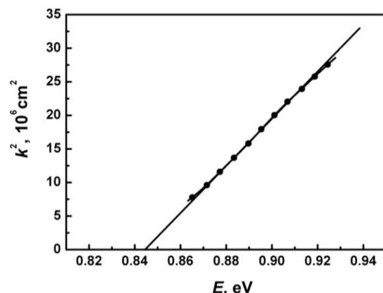
Fig. 2 – Spectral dependence of  $k^2$  for germanium film on gallium arsenide in the region of  $E_0$  transition
