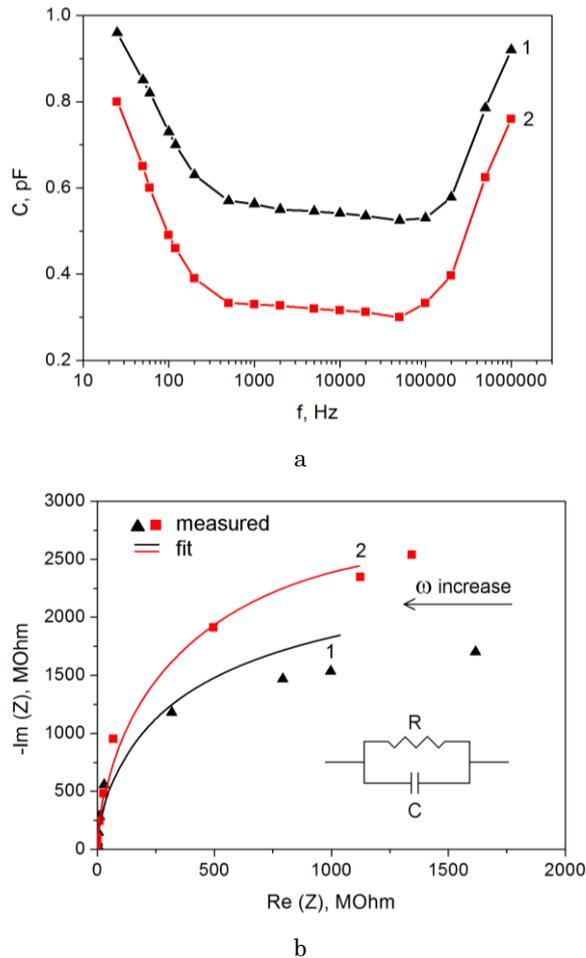
**Fig. 3** – Frequency dependences of electrical capacitance (a) and Nyquist plots (b) of the PS<sub>111</sub> (1) and PS<sub>100</sub> (2) nanosystems. Inset: equivalent circuit diagram of the PS-based nanosystems
