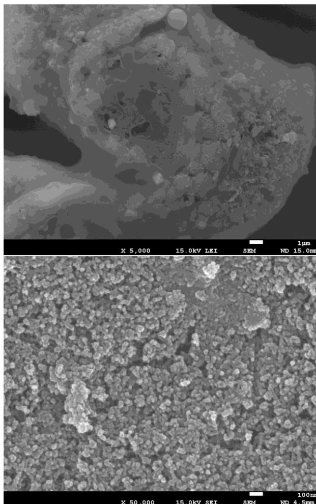
**Fig. 2** – SEM images of the PS<sub>100</sub> nanocrystals in the epoxy polymer at various magnifications
