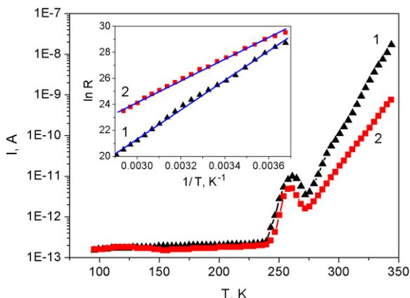
**Fig. 4** – Temperature dependences of conductivity current for the PS<sub>111</sub> (1) and PS<sub>100</sub> (2) nanosystems. Inset shows the same temperature dependences in  $\ln R-T^{-1}$  coordinates
