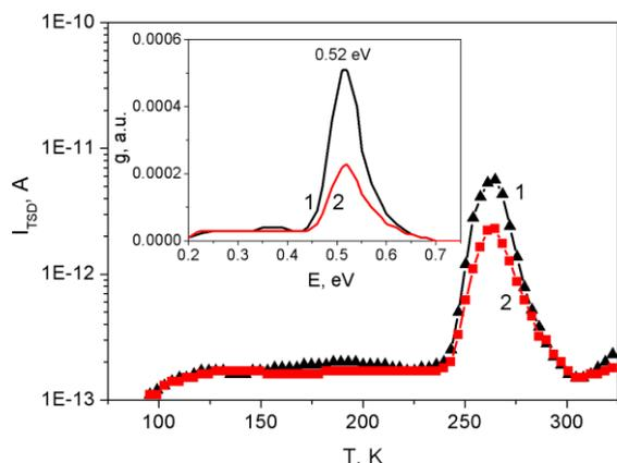
**Fig. 5** – Temperature dependences of depolarization current and energy distribution of the density of states (inset) in the PS<sub>111</sub> (1) and PS<sub>100</sub> (2) nanosystems
