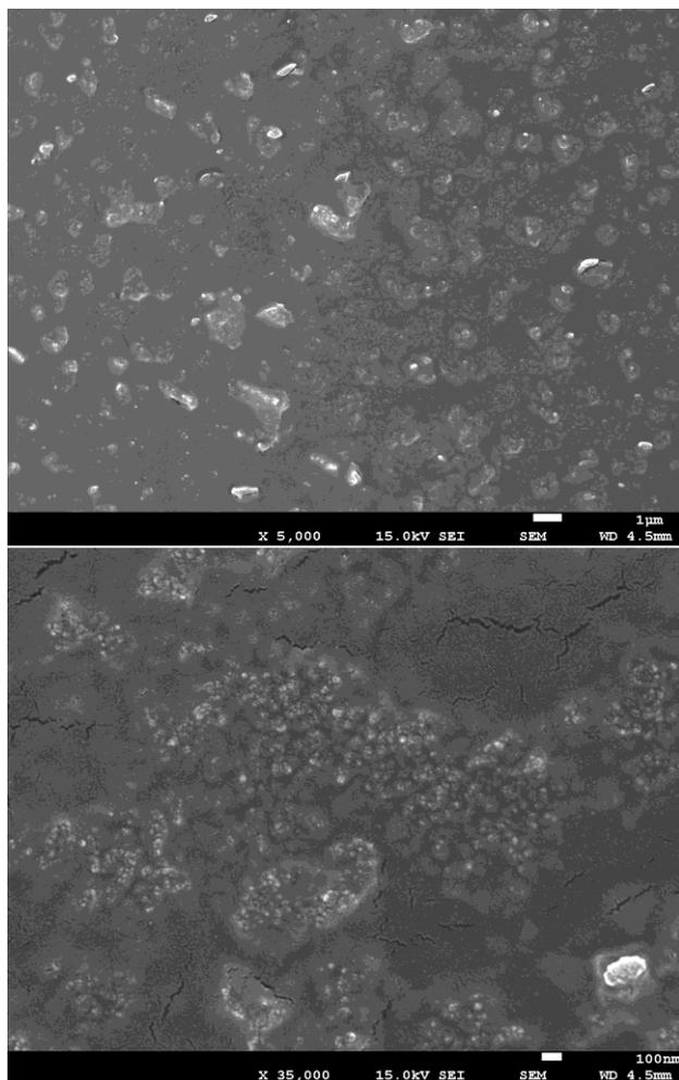
**Fig. 1** – SEM images of the PS<sub>111</sub> nanocrystals in the epoxy polymer at various magnifications
