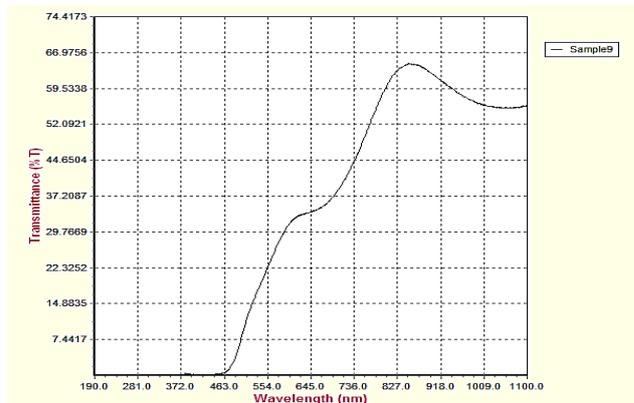
**Fig. 3 – Transmittance vs. wavelength (300 °C and 2 hours)**
