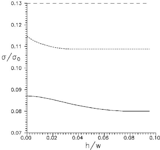
**Fig. 3** – Magnetic field dependences of conductivity for fixed values of band filling (semi-elliptic DOS,  $zJ_{eff}/w = 0$ ). The upper curve corresponds to  $n = 0.4$ ; middle curve  $n = 0.3$ ; the lower curve  $n = 0.2$
