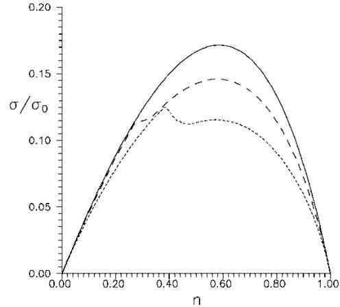
**Fig. 1** – Influence of the DOS form on the magnitude of the static conductivity at change of band filling. Solid curve corresponds to rectangular DOS, long-dashed curve corresponds to semi-elliptical DOS, short-dashed curve corresponds to DOS for sc-lattice
