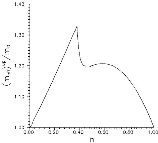
**Fig. 8** – Concentration dependence the effective mass for current carriers of spin  $\uparrow\uparrow$  for band filling interval  $n < 1$  at  $zJ_{eff}/w = 0$  in the absence of the correlated hopping for DOS of sc-lattice
