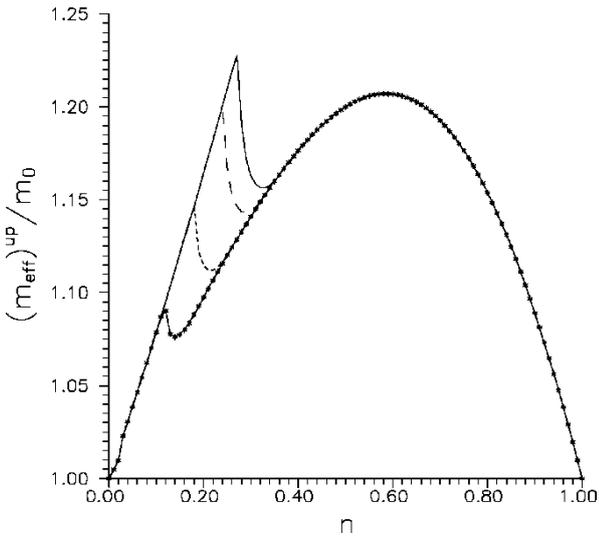
**Fig. 5** – Concentration dependence of the effective masses of current carriers with spin  $\downarrow\downarrow$  (upper curve) and  $\uparrow\uparrow$  (lower curve) at  $J_{eff}/w = 0$  in the absence of the correlated hopping for semi-elliptical DOS
