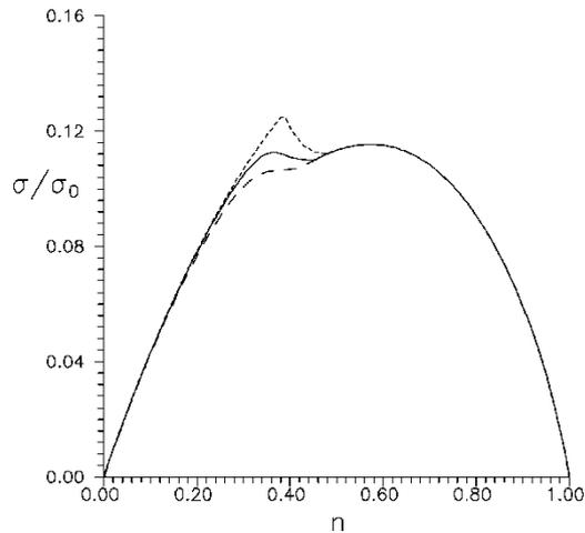
**Fig. 2** – Influence of magnetic field on concentration dependence of conductivity at DOS of sc-lattice. Short-dashed curve corresponds to  $h/w = 0$ ; solid curve –  $h/w = 0.03$ ; long-dashed curve –  $h/w = 0.06$
