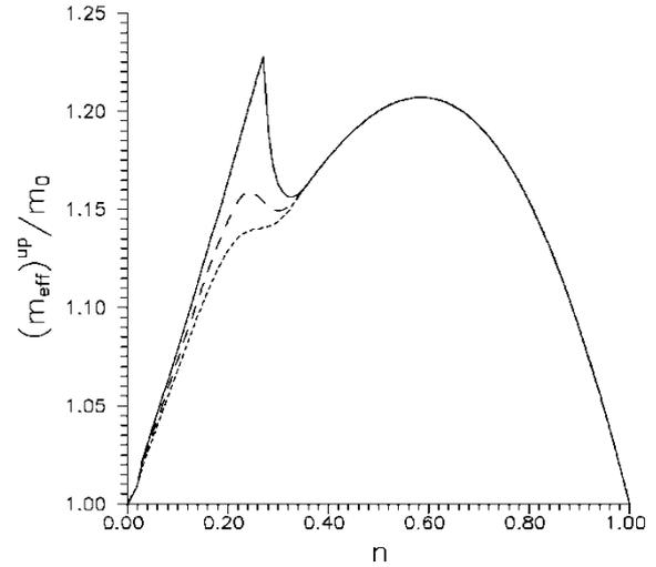
**Fig. 10** – Comparison of concentration dependences of effective masses of current carriers with spin in the absence (solid curve) or presence (long-dashed curve –  $h/w = 0.01$ , short-dashed curve –  $h/w = 0.02$ ) of magnetic field (semi-elliptic DOS,  $zJ_{eff}/w = 0$ ,  $\tau_1 = 0$ )
