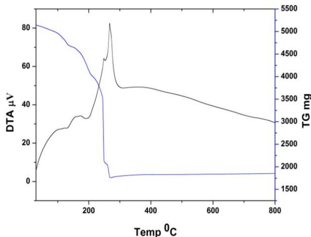
Fig. 6 – TG/DTA of CuO nanoparticles
