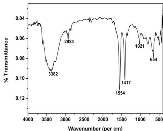
Fig. 2 – FTIR spectra of CuO nanoparticles
