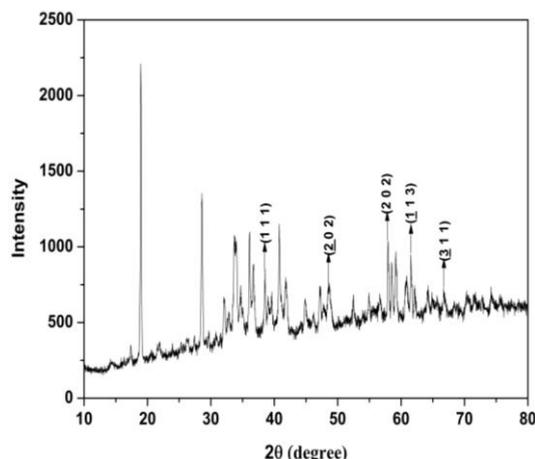
Fig. 1 – X-ray diffraction pattern of CuO nanoparticles
