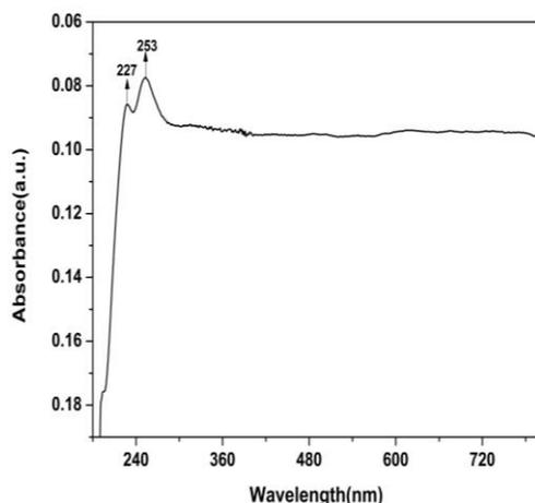
Fig. 4 – UV-visible spectra of CuO nanoparticles
