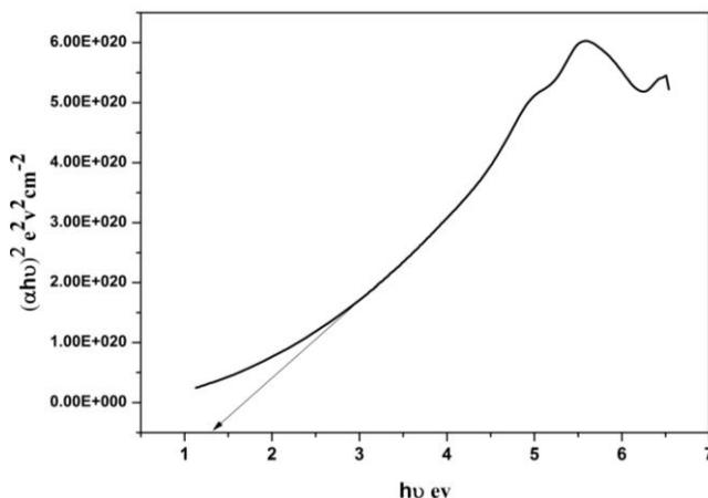
Fig. 5 – Band gap energy of CuO nanoparticles
