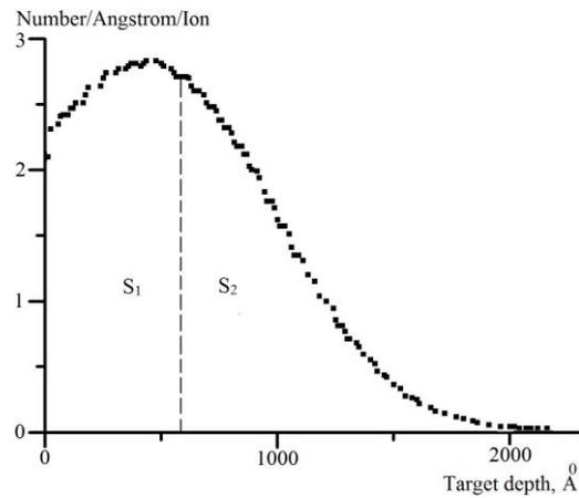
Fig. 6 – Distribution of vacancies that appeared by irradiation with  $\text{Cu}^{2+}$  ions of a copper surface with an initial energy of 300 keV based on the results of calculations of the program SRIM
