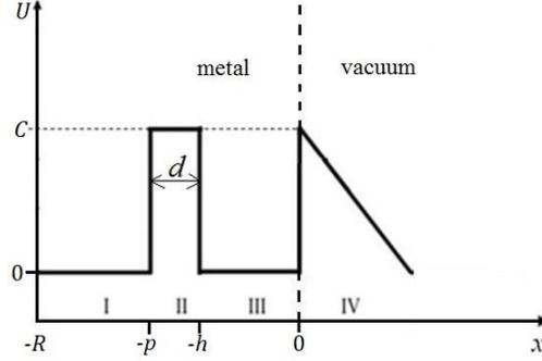
Fig. 1 – Diagram of the potential barrier for escape of electrons from the modified metal surface to vacuum
