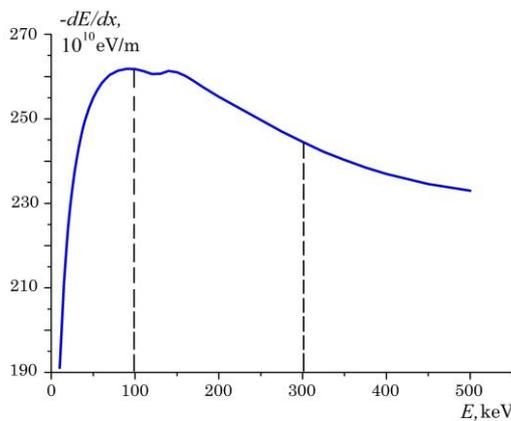
Fig. 5 – Graph of the dependence of the full stopping power of  $\text{Cu}^{2+}$  ions on energy in copper
