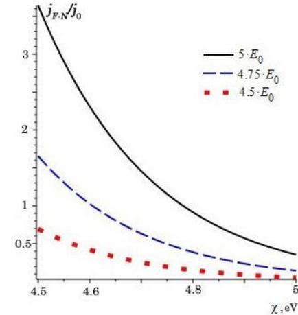
Fig. 4 – The dependence of the current density on the metal work function at different electric field strengths
