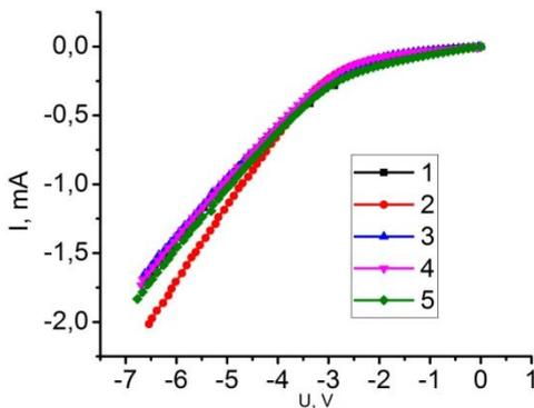
Fig. 3 – Volt-ampere characteristics of the sample when the electric current was in the opposite direction (red color - one hour after hydrogen processing)
