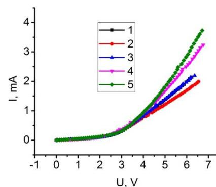
**Fig. 2** – Volt-ampere characteristics of the sample when the electric current was in the positive direction: 1) before hydrogen treatment; 2) one hour after hydrogen treatment; 3) 22 hours after hydrogen treatment; 4) three days after hydrogen treatment; 5) a week after hydrogen treatment
