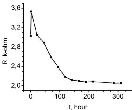
Fig. 4 – Time dependence of the sample electrical resistance after hydrogen treatment
