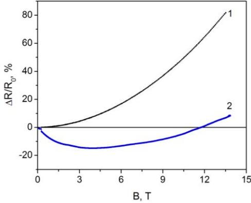
**Fig. 1** – Longitudinal magnetoresistance of Si whiskers at a temperature of 4.2 K for samples: 1 – unstrained; 2 – strained
