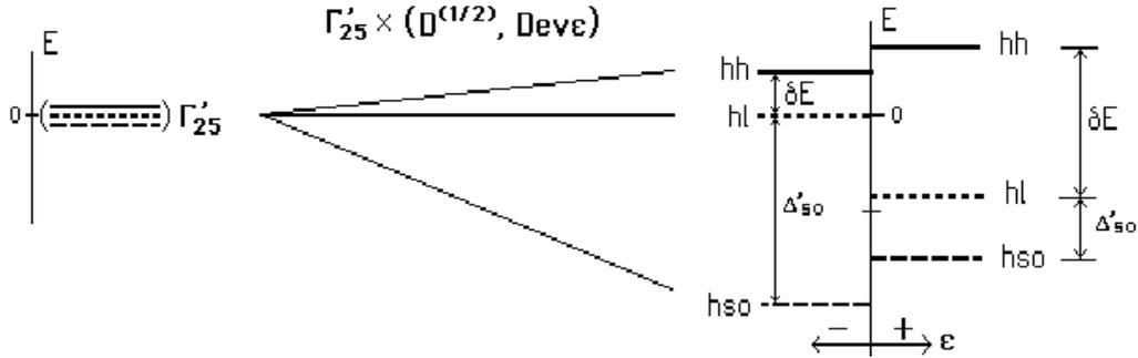
**Fig. 4** – The strain genesis of the valence band in a three-zone approximation
