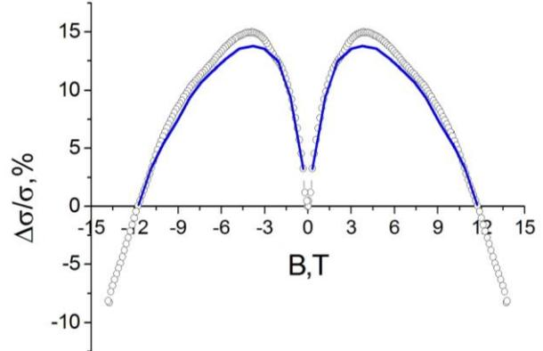
**Fig. 2** – Longitudinal magnetoconductance in Si whiskers at a temperature of 4.2 K. Solid line corresponds to the theoretical data, while circles denote experimental ones
