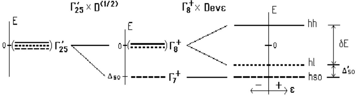
**Fig. 3** – The strain genesis of the valence band in a two-zone approximation
