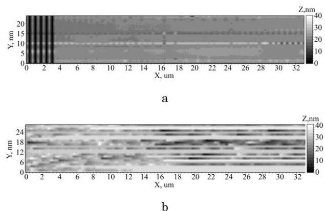
**Fig. 7** – The result of sclerometry of the silver coating surface obtained by combined precipitation in vacuum after electron beam modification (a) and coating obtained in the industrial process (b)
