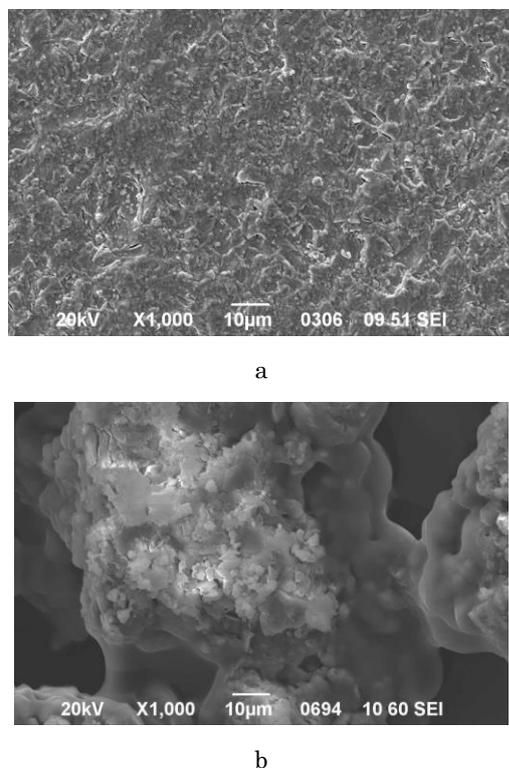
**Fig. 5** – Fragments of electrode surfaces on samples with piezoceramics PZT-5 (were in operation under extreme conditions for 10 years): (a) electrodes modified with an electron stream (I group of samples) (b) electrodes produced by industrial method (II group of samples). Device ZEISS EVO 50 XVP
