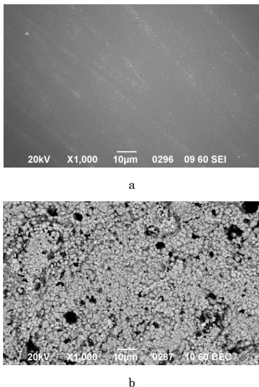
**Fig. 4** – Fragments of electrode surfaces on samples with piezoceramics PZT-5 (were not in operation): (a) electrodes modified with an electron stream (I group of samples); (b) electrodes produced in the industrial process (II group of samples). Device ZEISS EVO 50 XVP
