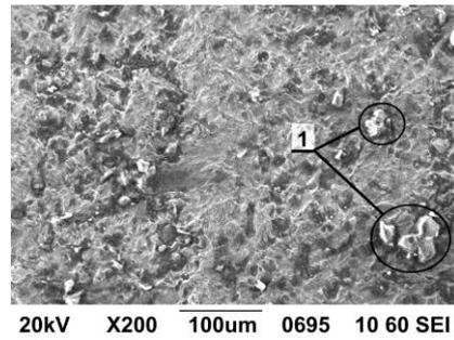
**Fig. 2** – The surface of the silver electrode of the sample from the piezoelectric ceramics PZT-5 with formed on it, due to electron-beam modification, at temperatures above 900 K, silver conglomerates (1). Device ZEISS EVO 50 XVP
