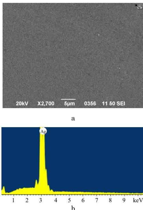
**Fig. 6** – Image of the surface of the sample of Group I after the electron-beam modification (a) and the energy spectrum of the distribution of chemical elements in the coating (b). Device ZEISS EVO 50 XVP, Increase  $\times 10000$
