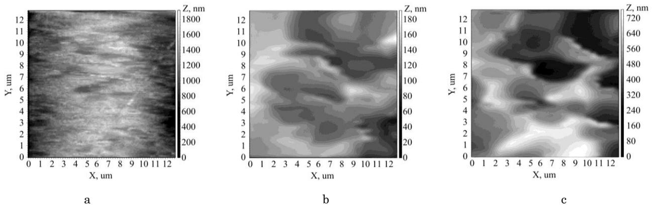
**Fig. 3** – The surface of the silver coating on piezoelectric ceramics PZT-5 of group II (a) and group I: with electron-beam modification at a temperature of 880 K (b) and with electron-beam modification at a temperature of 780 K (c). Device NT-206
