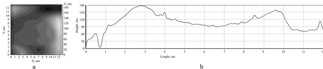
**Fig. 1** – External view (a) and microprofile of the surface of the silver electrode (b). Device NT-206
