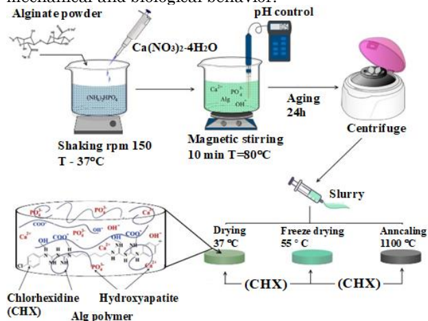
Fig. 6 – Scheme for the preparation of a HA/Alg/CHX composites [8]
