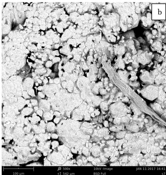
**Fig. 6** – Structure of PAN granule with an excessive humidity: a – abrading of the granule; b – dissolution of the granule part
