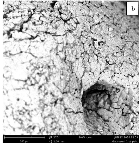
**Fig. 5** – Structure of the PAN granule, which is obtained after drying in the vortex granulator with drying overtime: a – cracks; b – partial destruction of the granule
