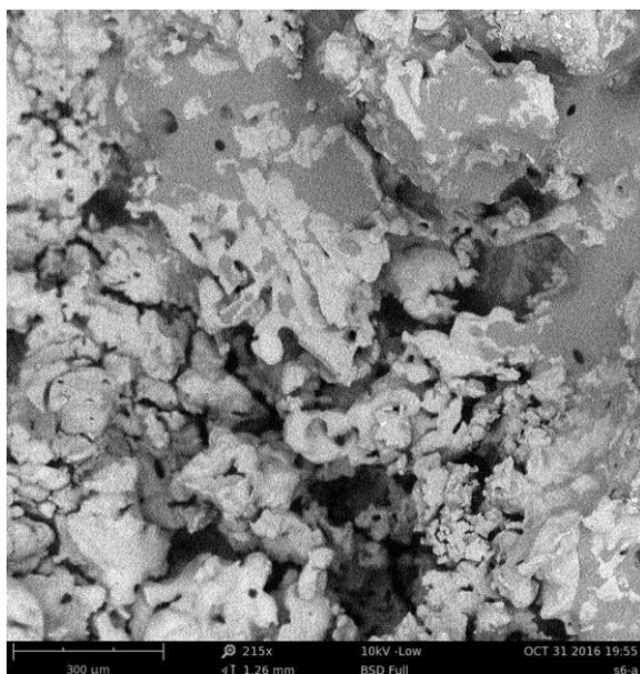
**Fig. 7** – Structure of the PAN granule after the finish drying stage in the gravitational shelf dryer
