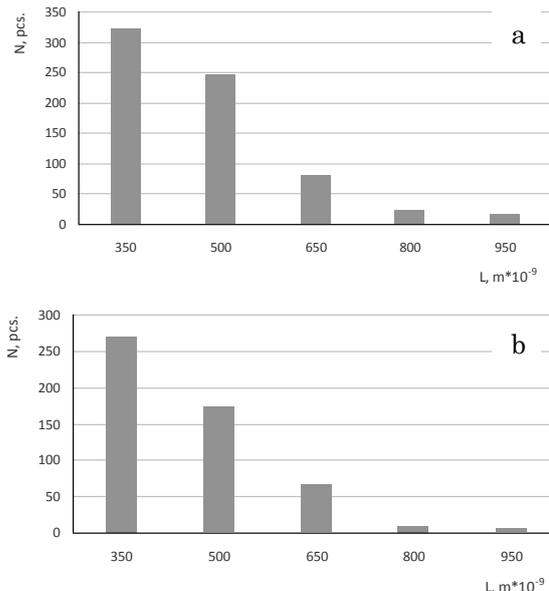
**Fig. 8** – Number and sizes of pores per unit of PAN granule surface area (granule, humidified with water): a – surface; b – subsurface layers
