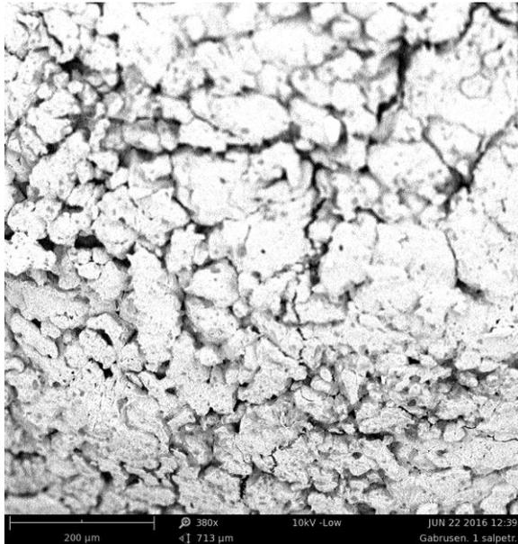
**Fig. 4** – Structure of PAN granule, which is obtained in the optimal regime of the granulator work
