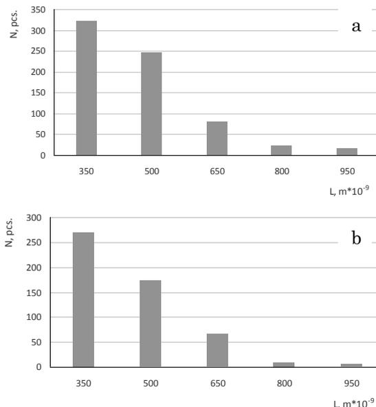
**Fig. 8** – Number and sizes of pores per unit of PAN granule surface area (granule, humidified with water): a – surface; b – subsurface layers
