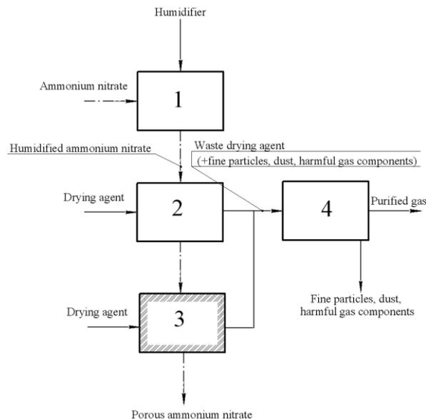
**Fig. 2** – Scheme of PAN obtaining process: 1 – humidification of ammonium nitrate granule; 2 – granulation-drying; 3 – finish drying; 4 – cleaning of waste gas
