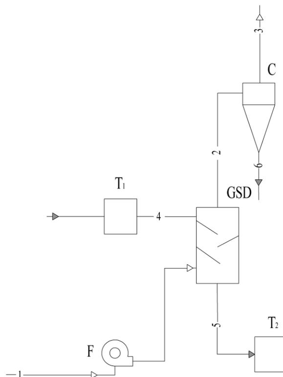
**Fig. 3** – Schematic diagram of the experimental setup for the study of shelf devices: F – fan; GSD – gravitational shelf unit; C – cyclone; T1, T2 – containers (tanks); 1 – drying agent; 2 – waste drying agent; 3 – purified gas; 4 – PAN; 5 – PAN after final drying; 6 – fine particles
