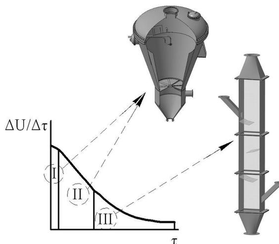
**Fig. 1** – Periods of PAN granule drying: I – warming-up of the granule; II – period of the drying constant velocity; III – period of the drying reducing velocity
