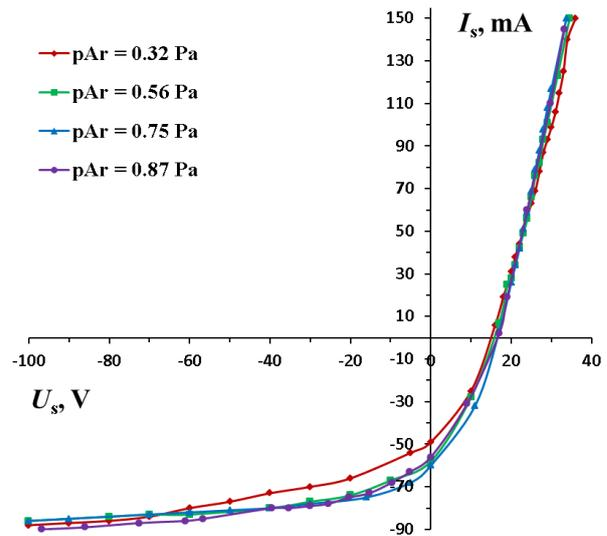
Fig. 2 – Current-voltage characteristics measured on the substrate at different pressures of the working gas. Negative semiaxis  $I_s$  corresponds to the ion current on the substrate, and the positive one to the electron
