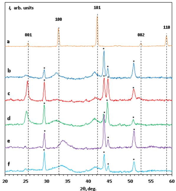
Fig. 3 – Diffraction patterns of hafnium diboride films obtained at different values of the substrate bias: a) target; b) – 50 V; c) – 25 V; d) 0 V (ground); e) +25 V; f) +50 V. The symbol “\*” indicate the reflexes of the substrate
