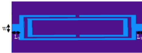
Fig. 5 – Bandstop filter topology using line loaded with RSRR
