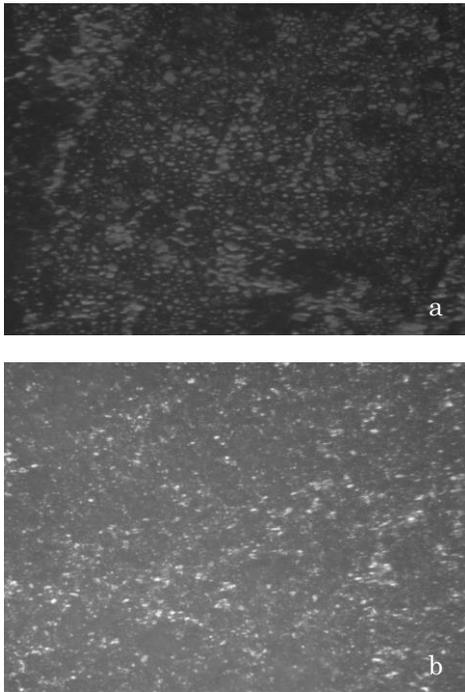
**Fig. 1** – Optical micrograph of Ni-Co ferrites: a –  $\text{CoFe}_2\text{O}_4$ , b –  $\text{Ni}_{0.5}\text{Co}_{0.5}\text{Fe}_2\text{O}_4$
