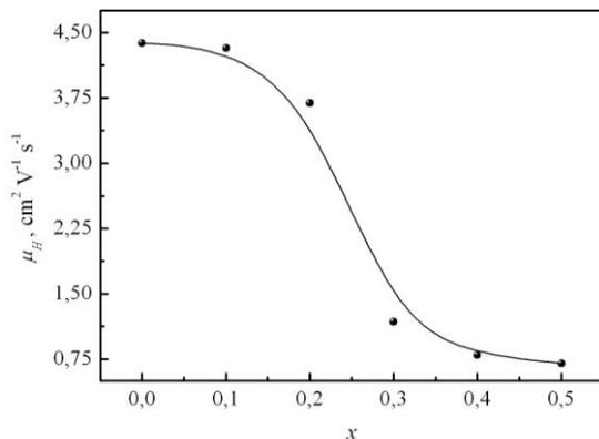
**Fig. 6** – The dependence of Hall mobility from content of  $\text{Ni}^{2+}$  ions
