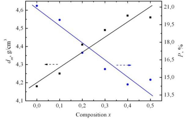
Fig. 4 – Dependences of relative density and porosity from content of  $\text{Ni}^{2+}$  ions
