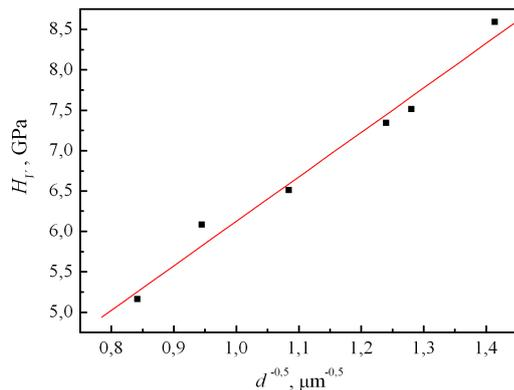
Fig. 3 – Hall-Petch plot for the Ni-Co ferrites
