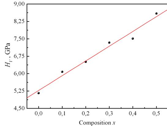
**Fig. 2** – The microhardness of  $\text{Ni}_x\text{Co}_{1-x}\text{Fe}_2\text{O}_4$  ferrites as a function of Ni content
