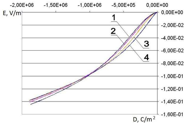
**Fig. 3** – Dependence of the electric displacement on the strength of the applied electric field (sample  $\text{Ba}_{0.75}\text{Sr}_{0.25}\text{Ti}_{0.95}\text{Zr}_{0.05}\text{O}_3$ ). 1 – 24 °C; 2 – 35 °C; 3 – 55 °C; 4 – 45 °C
