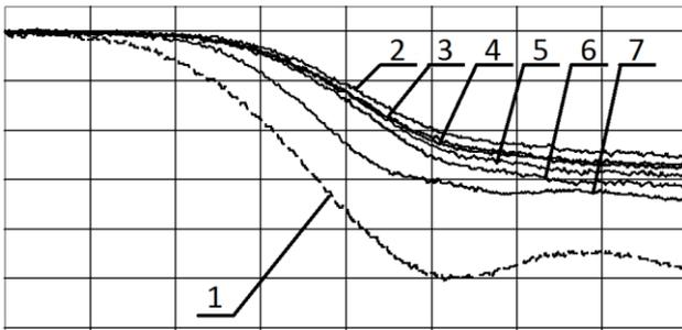
**Fig. 2** – Typical oscillograms ( $5 \cdot 10^{-8}$  s/div) of the EF strength and electric displacement in  $\text{Ba}_{0.75}\text{Sr}_{0.25}\text{Ti}_{0.95}\text{Zr}_{0.05}\text{O}_3$  ceramic samples. Curve 1 corresponds to EF strength ( $3.2 \cdot 10^5$  (V/m)/div); curves 2-7 correspond to electric displacement ( $4.29 \cdot 10^{-1}$  (C/m<sup>2</sup>)/div) in a sample at temperatures 25.8 °C, 30 °C, 35 °C, 40 °C, 45 °C, 55 °C correspondingly
