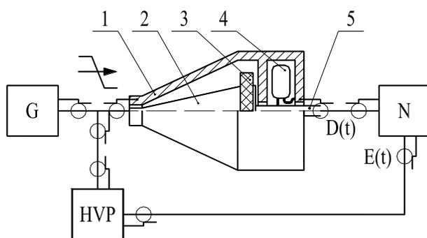
**Fig. 1** – Setup for synchronous oscilloscoping of electric field strength and electric displacement in ferroelectric ceramics samples at pulsed polarization. G is pulsed generator of monotonically increasing voltage; HVP is high voltage probe; N is two-channel oscilloscope; 1 is casing; 2 is high-voltage electrode; 3 is ferroelectric ceramics sample; 4 are measuring capacitors; 5 is intermediate electrode, output of  $D(t)$  channel
