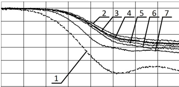
**Fig. 2** – Typical oscillograms ( $5 \cdot 10^{-8}$  s/div) of the EF strength and electric displacement in  $\text{Ba}_{0.75}\text{Sr}_{0.25}\text{Ti}_{0.95}\text{Zr}_{0.05}\text{O}_3$  ceramic samples. Curve 1 corresponds to EF strength ( $3.2 \cdot 10^5$  (V/m)/div); curves 2-7 correspond to electric displacement ( $4.29 \cdot 10^{-1}$  (C/m<sup>2</sup>)/div) in a sample at temperatures 25.8 °C, 30 °C, 35 °C, 40 °C, 45 °C, 55 °C correspondingly
