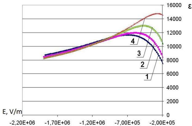
**Fig. 4** – Dependence of the dielectric permittivity on the electric field strength (sample  $\text{Ba}_{0.75}\text{Sr}_{0.25}\text{Ti}_{0.95}\text{Zr}_{0.05}\text{O}_3$ ). 1 – 24 °C; 2 – 35 °C; 3 – 55 °C; 4 – 45 °C
