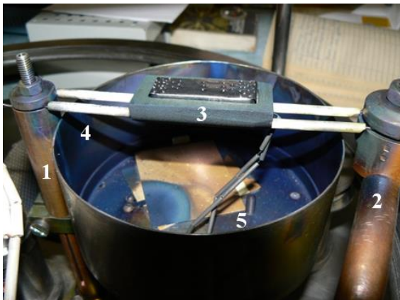
Fig. 1 – Graphite evaporator of cadmium telluride: 1, 2 – current inputs; 3 – graphite crucible with a hole cricket; 4 – heating elements; 5 – thermocouple
