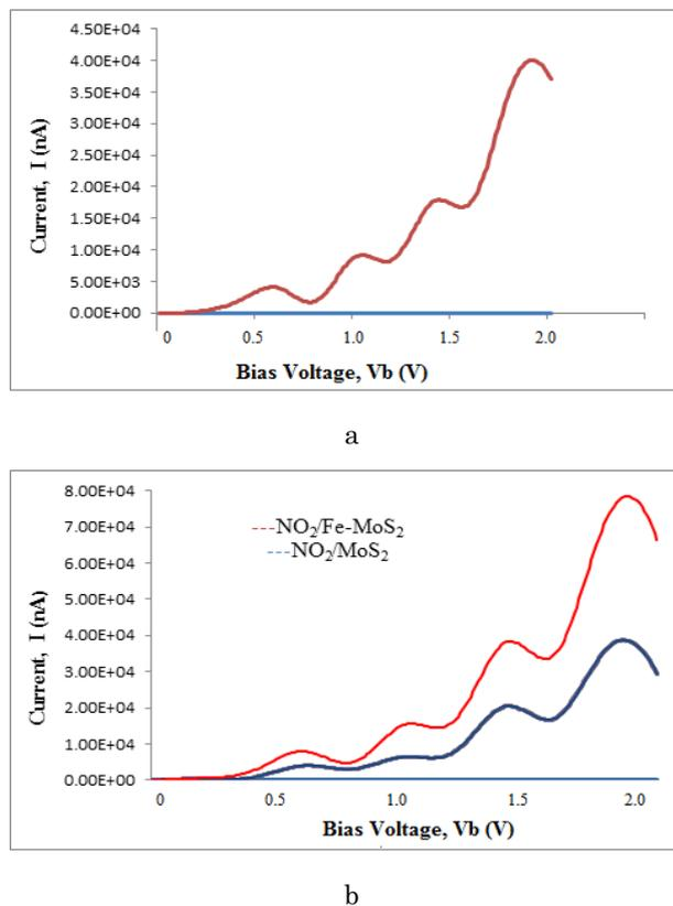
Fig. 2 –  $I$ - $V$  curves of the MoS<sub>2</sub> (a),  $I$ - $V$  curves of the NO<sub>2</sub>-MoS<sub>2</sub> and NO<sub>2</sub>/Fe-MoS<sub>2</sub> (b)
