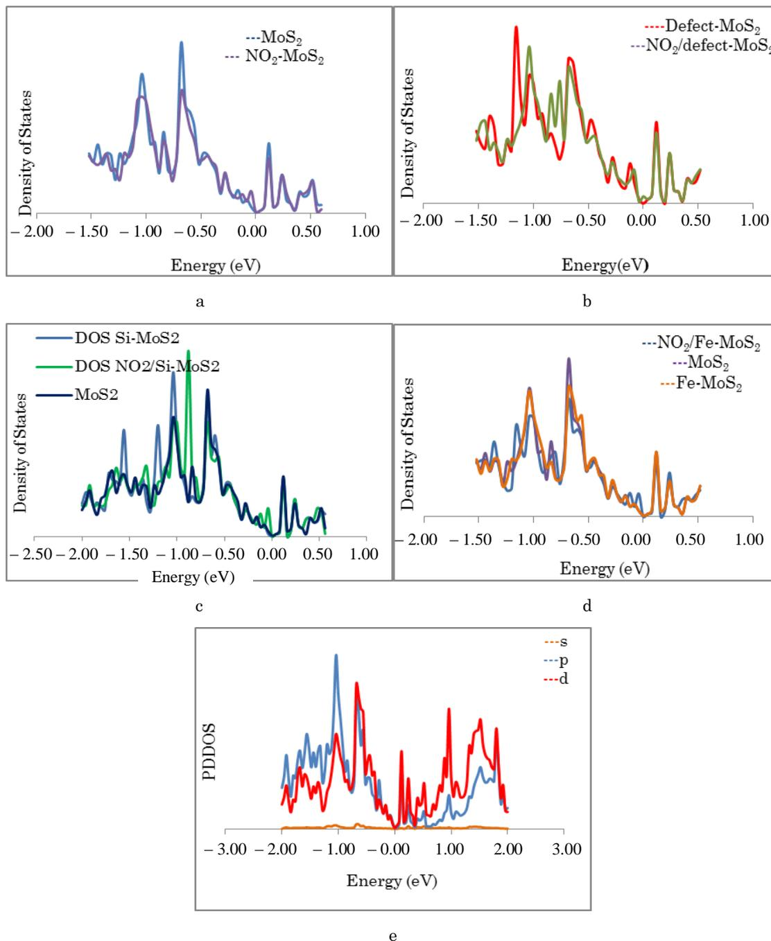
**Fig. 1** – DOS of MoS<sub>2</sub> and NO<sub>2</sub>-MoS<sub>2</sub> (a), DOS of defect-MoS<sub>2</sub> and NO<sub>2</sub>/defect-MoS<sub>2</sub> (b), The spin-up electronic density of states for pristine, Si-MoS<sub>2</sub> and NO<sub>2</sub>/Si-MoS<sub>2</sub>(c), The spin-up electronic density of states for pristine, Fe-MoS<sub>2</sub> and NO<sub>2</sub>/Fe-MoS<sub>2</sub> (d), The PDOS of Fe in Fe-MoS<sub>2</sub> (e)
