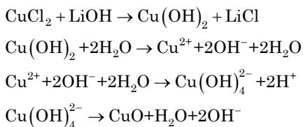
In reaction between  $\text{CuCl}_2$  and  $\text{LiOH}$  in aquatic media,  $\text{Cu(OH)}_2$  is formed initially which further produces  $\text{Cu(OH)}_4^{2-}$ . At the onset of saturation  $\text{CuO}$  nuclei are formed and grow up to form the nanoparticles. The basic form of  $\text{Cu(OH)}_2$  and  $\text{CuO}$  are shown in Fig. 2 and Fig. 3 respectively.
