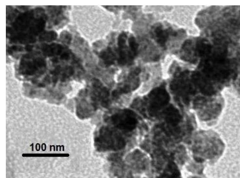
**Fig. 1** – TEM image of CuO nanoparticles dispersed on carbon coated copper grid
