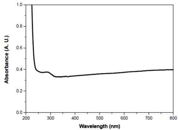
**Fig. 4 – UV-visible spectrum of Copper Oxide nanoparticles**
