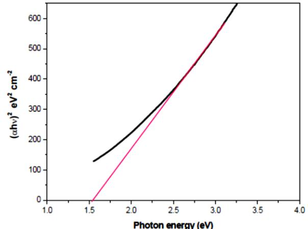
**Fig. 5 – Plot from UV-VIS data to determine band gap of synthesized copper oxide**
