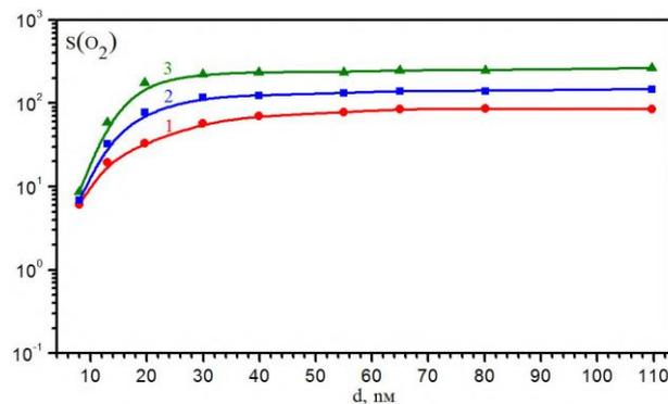
Fig. 5 – Dependence of the magnitude of the sensory signal  $S(O_2)$  of nanopowder ZnO (initial (1), Al (3 at.%) doped (2) and laser annealed (3) ( $E_i = 0.22 \text{ J/cm}^2$ ,  $\tau = 10 \text{ ns}$ )) of the size of the nanoparticless ( $d$ )
