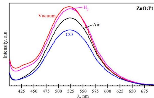
**Fig. 3** – Photoluminescence spectra of ZnO:Pt in various gas environments
