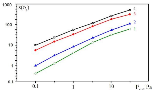
Fig. 4 – Dependence of the sensory signal value  $S(O_2)$  of ZnO nanopowders (1 – ZnO, 2 – ZnO:Ag, 3 – ZnO:Au, 4 – ZnO:Pt) from the additional partial pressure of oxygen in the air
