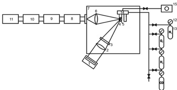
**Fig. 1** – Scheme of the installation for studying the photoluminescence properties of nanopowders in gases: 1 – UV source; 2, 6 – lens; 3 – optical filter UFS-2; 4 – quartz cell; 5 – sample; 7 – light-defensive camera; 8 – monochromator DMR-4; 9 – photomultiplier FEU-27; 10 – amplifier; 11 – PC; 12 – vacuum gauge IV-2; 13 – gas bottle; 14 – active volume; 15 – vacuum assembly VUP-5M
