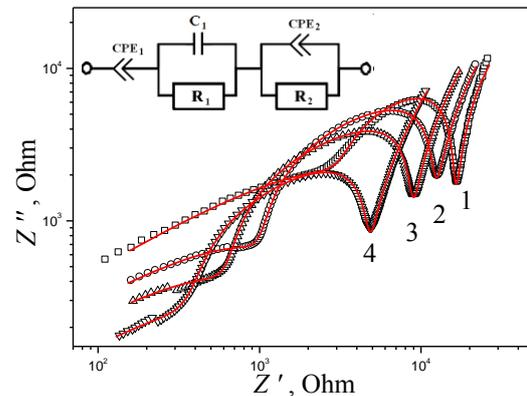
**Fig. 5** –  $Z'-Z''$  diagrams for the systems based on PPG, which filled by MWCNTs: 1 – 0.4 %; 2 – 0.5 %; 3 – 0.6 %; 4 – 0.7 %. Empty symbols are the experimental data, a solid line is a model
