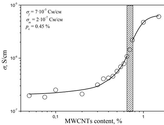
**Fig. 3** – Dependence of conductivity on MWCNTs content. Circles indicate an experimental data, solid line is the McLachlan model, dashed area is the area of the percolation threshold
