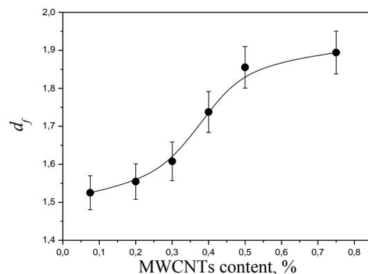
Fig. 2 – Dependence of fractal dimension on MWCNTs content
