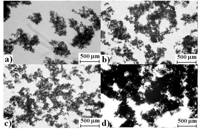
Fig. 1 – The microscopic images of the system based on PPG and MWCNTs. MWCNTs content: a) 0.1 %; b) 0.3 %; c) 0.45 %; d) 0.75 %
