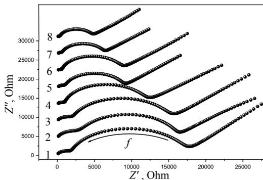
**Fig. 4** – Nyquist plots ( $Z''(Z')$  dependences) for the PPG-MWCNTs systems, where the MWCNTs content is: 1 – 0.35 %; 2 – 0.4 %; 3 – 0.45 %; 4 – 0.5 %; 5 – 0.55 %; 6 – 0.6 %; 7 – 0.65 %; 8 – 0.7 %
