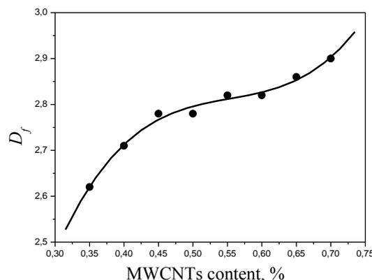
Fig. 6 – A value of fractal dimension of boundary layers for the PPG–MWCNTs systems, calculated using eq. (8)
