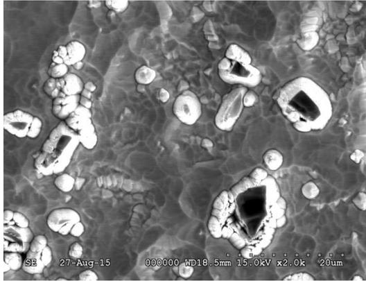
**Fig. 4** – SEM image of the surface processed mechanically during cutting of the PbTe crystal after sputtering by Ar plasma with 350 eV ions energy during 50 minutes
