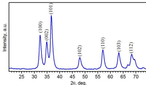
**Fig. 2** – XRD pattern ZnO nanopowders
