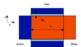
Fig. 1 – A GaSb-InAs Heterojunction Gate All Around TFET
