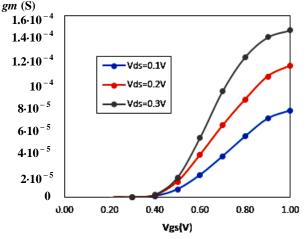
Fig. 3 – Transconductance at  $L_g = 22$  nm,  $N_d = 10^{18}$ /cm<sup>3</sup>
