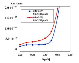
Fig. 4 – Gate-drain capacitance at  $L_g = 22$  nm, with  $N_d = 10^{18}/\text{cm}^3$  and  $10^{19}/\text{cm}^3$
