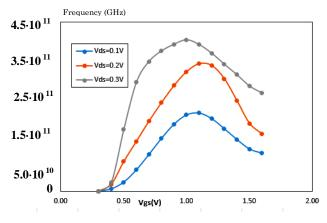
Fig. 6 – Cut-off frequency at  $L_g = 22$  nm,  $N_d = 10^{18}$ /cm<sup>3</sup>
