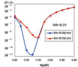
Fig.  $2 - I_d$ - $V_g$  characteristics at  $L_g = 22$  nm, with  $N_d = 10^{18}$ /cm<sup>3</sup> and  $10^{19}$ /cm<sup>3</sup>
