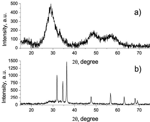
Fig. 1 – X-ray diffraction patterns of the samples obtained at the electrolyte temperature of 25 °C (a) and 98 °C (b)
