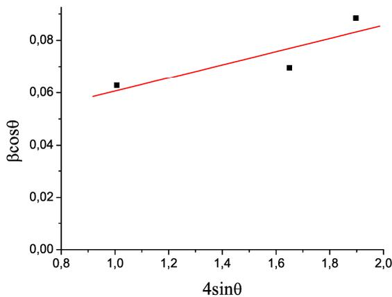
Fig. 3 – The use of the Williamson-Hall method for the determination of the contributions of the size effect and mechanical stresses for zinc sulfide
