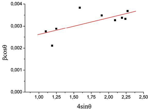
Fig. 2 – The use of the Williamson-Hall method for the determination of the contributions of the size effect and mechanical stresses for zinc oxide
