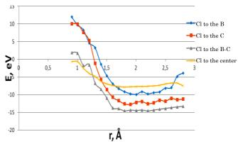
Fig. 4 – Profiles of the potential energy surface of interaction Cl atoms with the boron-carbon nanotube  $(6,\ 6)$  surface for four variants of atom orientation relative to boron-carbon tubulene
