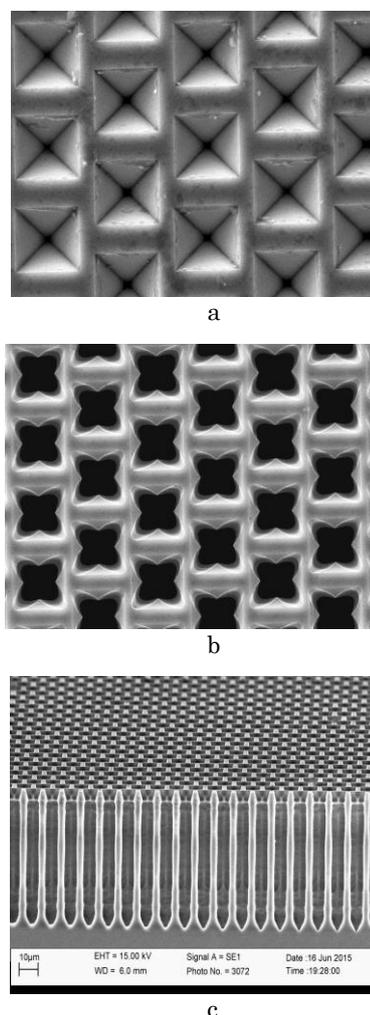
**Fig. 1** – SEM image of a silicon structure of BVC. a) type surface of the plates before deep anodic etching. Cellular location of the nucleation centers of pore growth, b) image of the surface after a deep anodic etching, c) image arbitrary cleavage of the MCS
