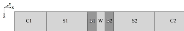
Fig. 2 – Schematic cross-sectional view of RTD, C1: Contact1, C2: Contact2, S1: Spacer1, S2: Spacer2, B1: Barrier1, B2: Barrier2, W: Well
