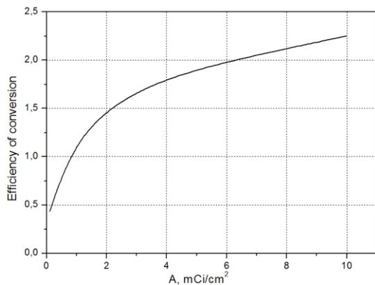
Fig. 8 – Dependence of the conversion efficiency of  $^{63}\text{Ni}$  radionuclide activity
