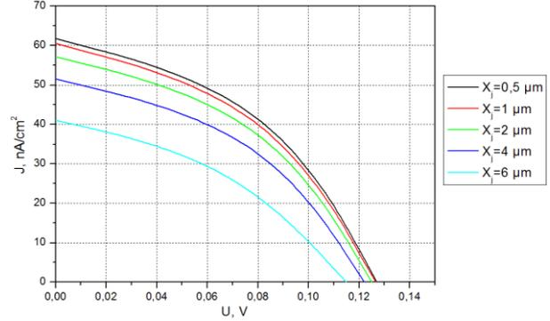
Fig. 2 – The dependence of the generated current in the structure vs voltage
