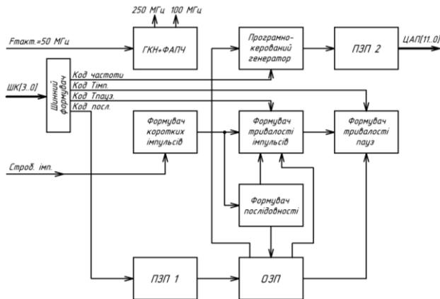
**Fig. 2** – Structural scheme of the imitation model of the digital processing core
