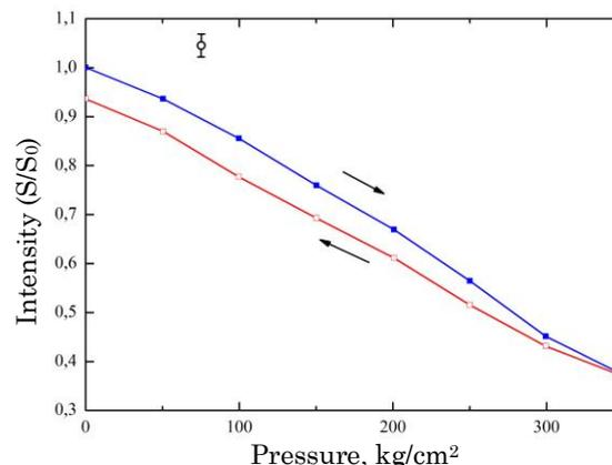
Fig. 8 – Dependence of the peak intensity of the resonance “a” line for the NQR spectrum of  $^{69}\text{Ga}$  in GaSe with increasing and decreasing pressure on the sample
