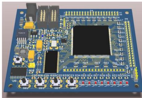
**Fig. 3** – Digital processing core of the experimental facility of the pulse method of NQR observation implemented on PLIC EP1C6Q240C8
