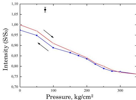
**Fig. 9** – Dependence of the peak intensity of the resonance “a” line for the NQR spectrum of  $^{115}\text{In}$  in InSe with increasing and decreasing pressure on the sample
