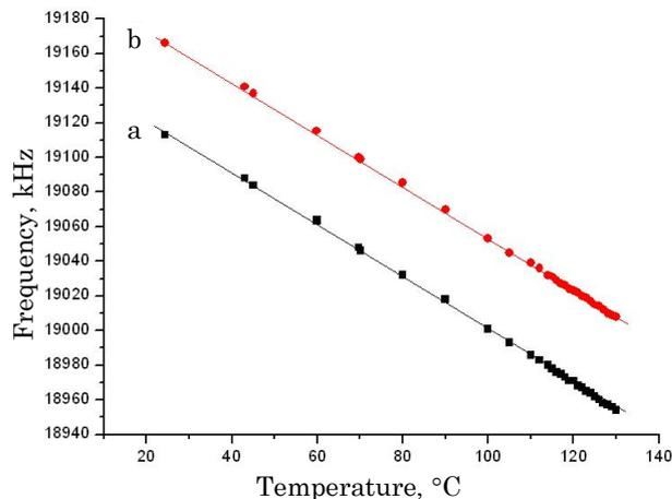
Fig. 6 – Frequency-temperature transformation obtained for the NQR spectrum of  $^{69}\text{Ga}$  in GaSe
