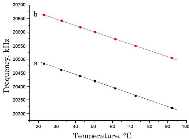
Fig. 7 – Frequency-temperature transformation obtained for the NQR spectrum of  $^{115}\text{In}$  in InSe
