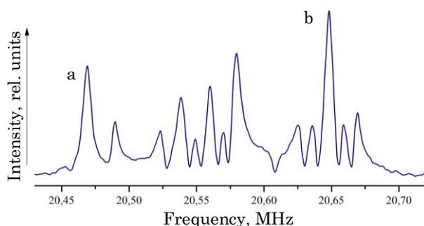
Fig. 5 – Experimental NQR spectrum of  $^{115}\text{In}$  in InSe for the spin transition on the frequency of 20.5 MHz
