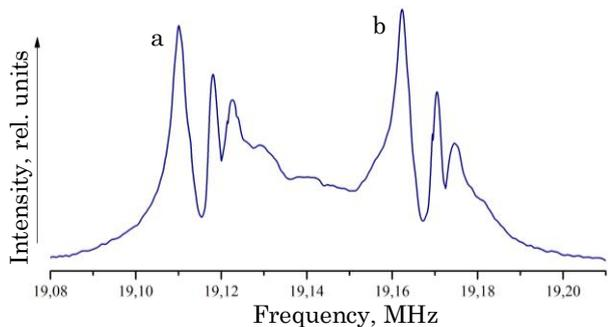
Fig. 4 – Experimental NQR spectrum of  $^{69}\text{Ga}$  in GaSe
