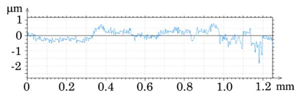
**Fig. 5** – Profilogram of the surface of the coatings of b series, covered with the coating (Zr-Ti-Nb)N ( $R_a = 0.42 \mu\text{m}$ )
