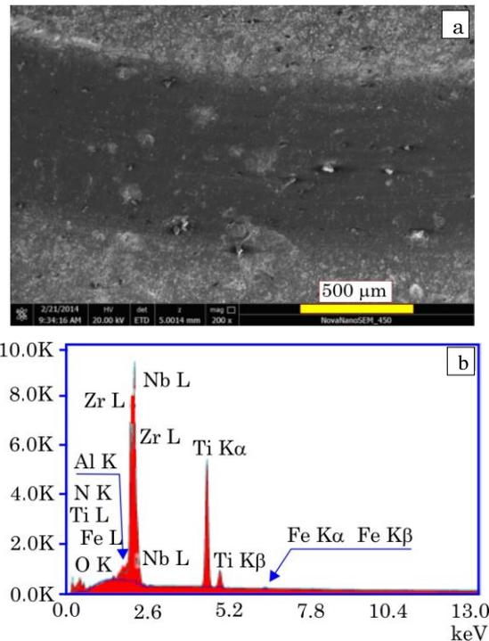
**Fig. 6** – Image of the surface of the sample of a series of (Zr-Ti-Nb)N system after the tests: a – general view of the surface of the coating with the wear track, b – chemical composition of the wear track
