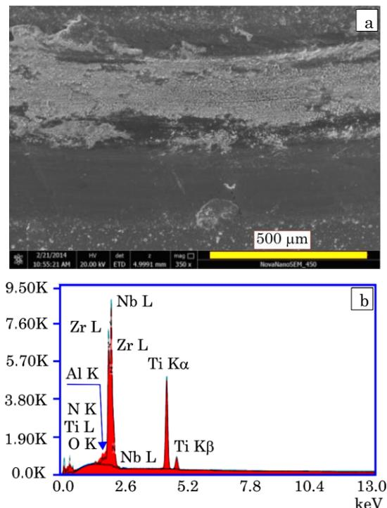
**Fig. 7** – Image of the surface of the sample of b series of (Zr-Ti-Nb)N system after the tests: a – general view of the surface of the coating with the wear track, b – chemical composition of the wear track
