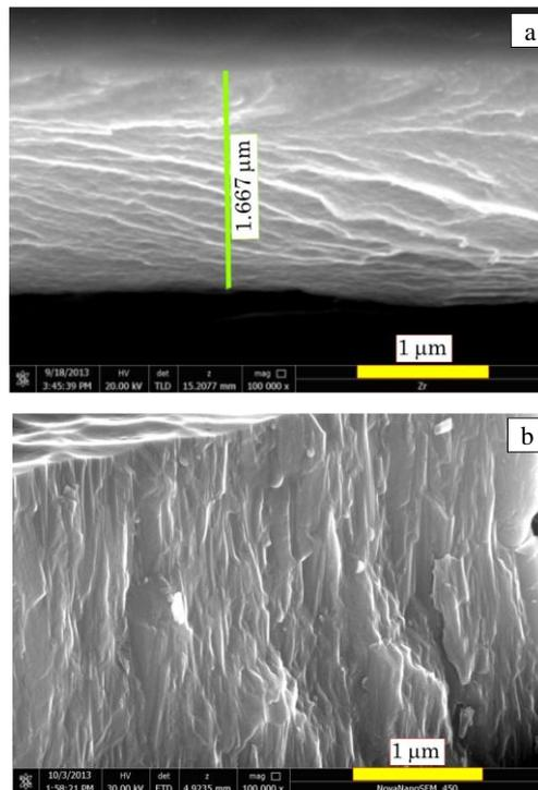
**Fig. 2** – Image of the fractograms of the fracture of the coatings (Ti-Zr-Nb)N, obtained at different partial pressures of nitrogen: *a* –  $P = 3 \times 10^{-4}$  Torr.; *b* –  $P = 4 \times 10^{-3}$  Torr
