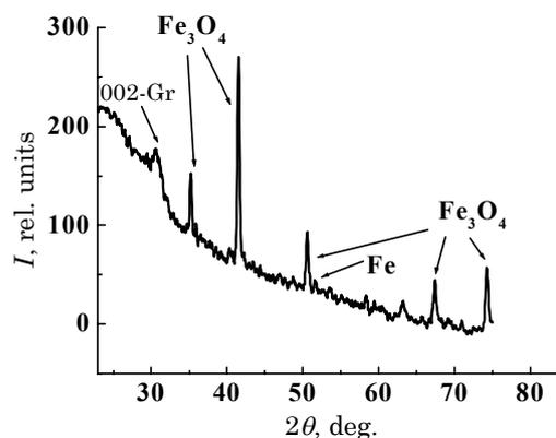
Fig. 2 – Fragment of the diffraction pattern of modified CNT
