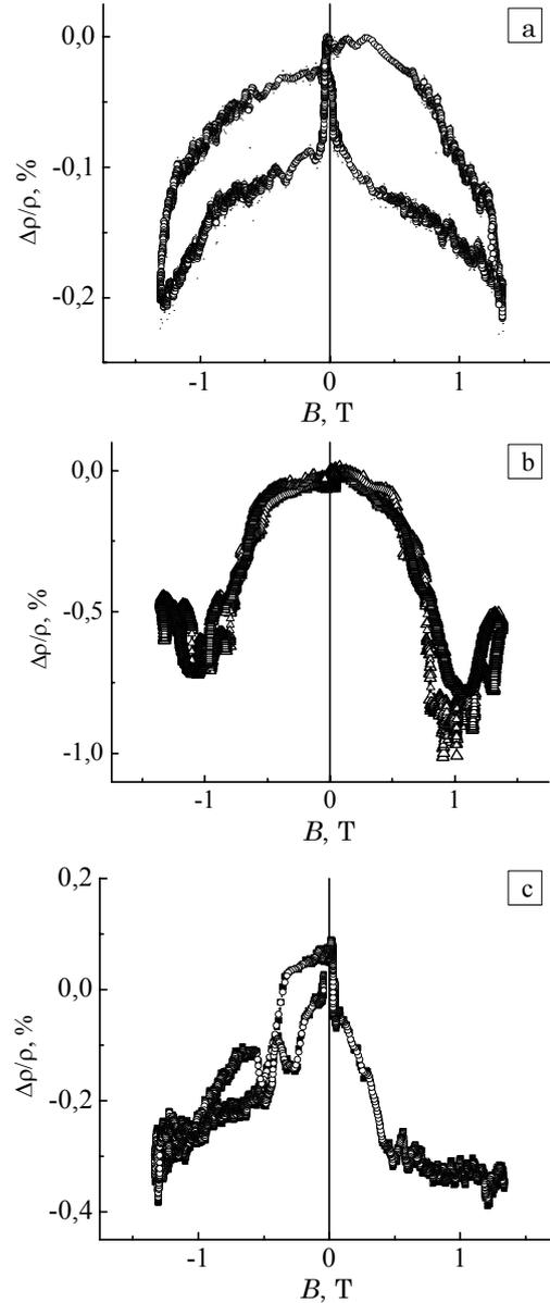
**Fig. 5** – Dependence of the magnetoresistance of modified CNT on the magnetic induction for  $B \perp I$  geometry at: (a)  $T = 293$  K, (b)  $T = 77$  K; for  $B \parallel I$  (c)  $T = 77$  K
