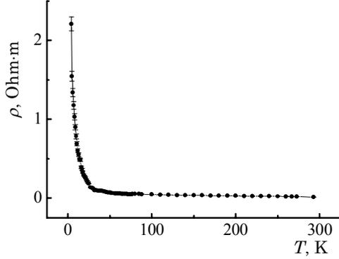
Fig. 3 – Temperature dependence of the electrical resistance of modified multi-walled CNT
