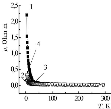
**Fig. 4** – Calculated dependences of the components  $\rho(T)$  according to the formula (1) for modified CNT (curve 1 – experimental values of  $\rho$ , curve 2 –  $C_3\rho_3$ , curve 3 –  $C_2\rho_2$ , 4 – theoretically calculated values of  $\rho$ )
