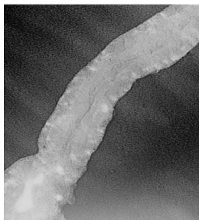
Fig. 1 – Electron-microscope image of a CNT modified by iron
