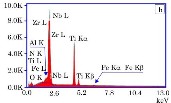
**Fig. 6** – Image of the surface of the sample of a series of (Zr-Ti-Nb)N system after the tests: a – general view of the surface of the coating with the wear track, b – chemical composition of the wear track
