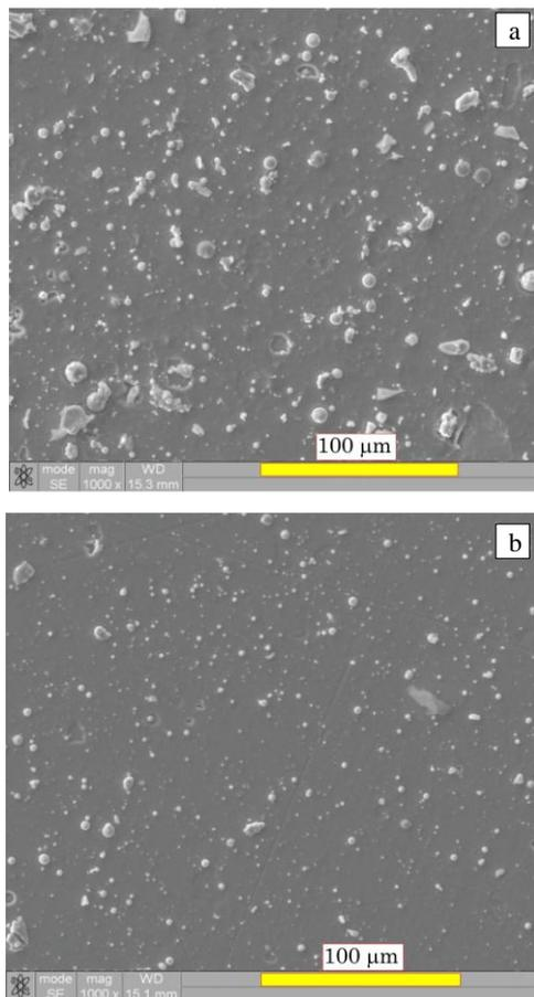
**Fig. 1** – Image of the surface of the coatings (Ti-Zr-Nb)N, obtained under different partial pressures:  $a - P = 3 \times 10^{-4}$  Torr ( $R_a = 1.17 \mu\text{m}$ );  $b - P = 4 \times 10^{-3}$  Torr ( $R_a = 0.42 \mu\text{m}$ )
