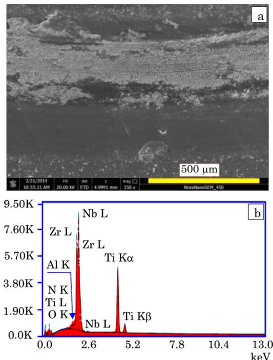
**Fig. 7** – Image of the surface of the sample of *b* series of (Zr-Ti-Nb)N system after the tests: *a* – general view of the surface of the coating with the wear track, *b* – chemical composition of the wear track
