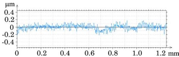
**Fig. 4** – Profilogram of roughness of the surface of steel disc after polishing ( $R_a = 0.088 \mu\text{m}$ )
