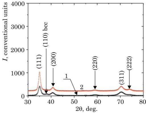
**Fig. 3** – X-ray diffraction spectra parts of the coatings obtained at different partial pressures of nitrogen: curve 1 –  $P = 3 \cdot 10^{-4}$  Torr; 2 –  $P = 4 \cdot 10^{-3}$  Torr
