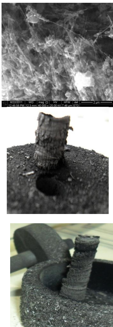
Fig. 1 – The deposit growth in the flat and hollow cathode and multiwall nanotubes contained in the central part of the deposit
