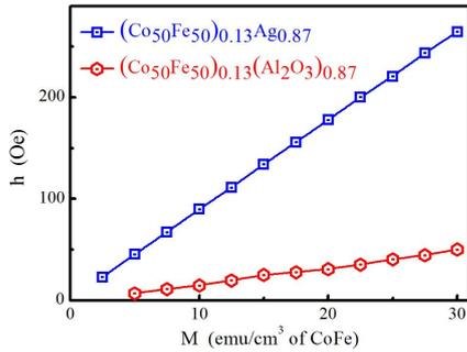
**Fig. 3** – Dependences of the effective values of indirect exchange interaction fields  $h_{\text{eff}}$  on the magnetization  $M$  for metal  $(\text{Co}_{50}\text{Fe}_{50})_{0.13}\text{Ag}_{0.87}$  and metal-dielectric  $(\text{Co}_{50}\text{Fe}_{50})_{0.13}(\text{Al}_2\text{O}_3)_{0.87}$  films
