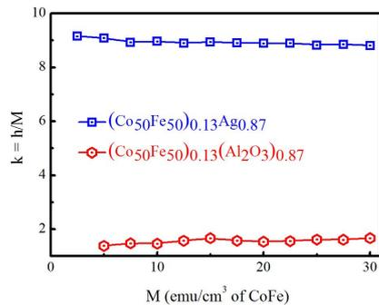
**Fig. 4** – Dependences of the indirect exchange interaction constant  $k$  on the magnetization  $M$  for metal  $(\text{Co}_{50}\text{Fe}_{50})_{0.13}\text{Ag}_{0.87}$  and metal-dielectric  $(\text{Co}_{50}\text{Fe}_{50})_{0.13}(\text{Al}_2\text{O}_3)_{0.87}$  films
