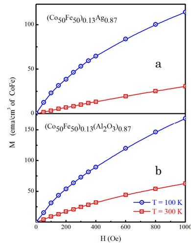
**Fig. 2** – Low-field parts of the magnetization curves for metal  $(\text{Co}_{50}\text{Fe}_{50})_{0.13}\text{Ag}_{0.87}$  (a) and metal-dielectric  $(\text{Co}_{50}\text{Fe}_{50})_{0.13}(\text{Al}_2\text{O}_3)_{0.87}$  (b) nanogranular films measured at 100 K and 300 K
