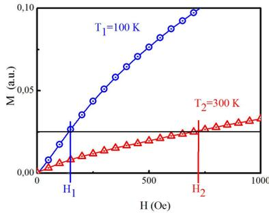
**Fig. 1** – Scheme for the calculation of the effective value of indirect exchange field  $h_{eff}$  in magnetic nanogranular films
