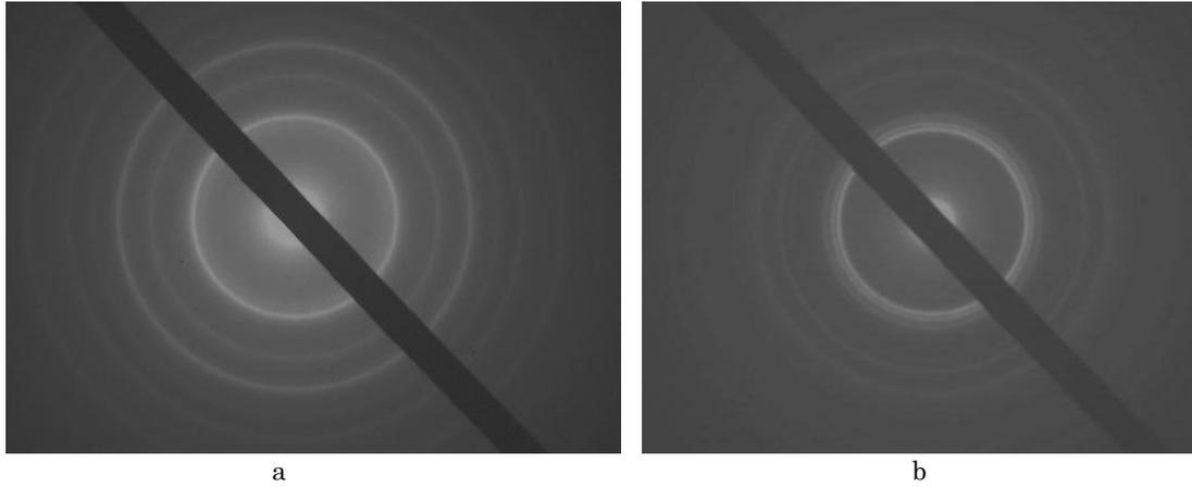
**Fig. 3** – Electron diffraction pattern from film system  $Fe(30) / Pt(15) / Fe(30) / S$ : a – non-annealing state (phase s.s. ( $\alpha$ -Fe)); b – after annealing to 800K (phase s.s. ( $\alpha$ -Fe) +  $Fe_3Pt$ ). Total concentration  $c_{Pt} \cong 20$  at. %
