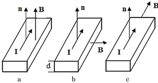
**Fig. 2** – Geometry measurement of MR: a – perpendicular ( $\perp$ ); b – transverse ( $\dagger$ ); c - longitudinal ( $\parallel$ ) geometry
