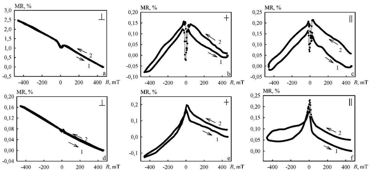
**Fig. 7** – The dependence MR versus magnetic field induction for non-annealing (a-c) and annealing from 800 K (d-f) film system [Fe(5) / Pt(5)Fe(5)]<sub>s</sub> / S. Temperature of measurement  $T = 300$  K
