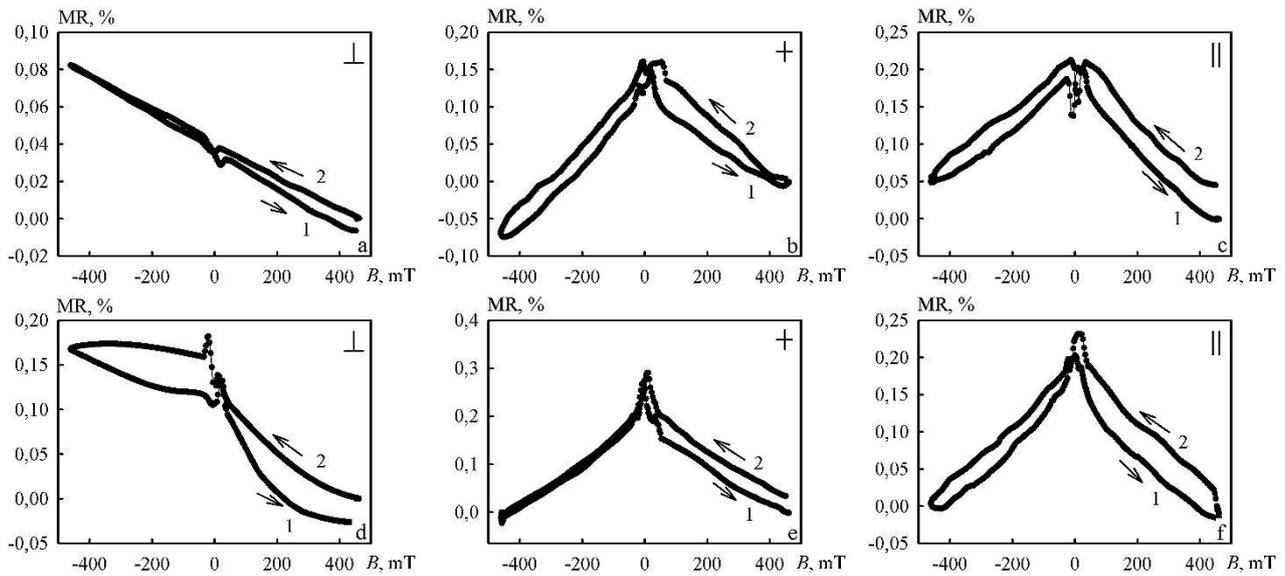
**Fig. 6** – The dependence MR versus magnetic field induction for non-annealing (a-c) and annealing from 800 K (d-f) film system [Fe(3) / Pt(3) / Fe(3)]<sub>s</sub> / S. Temperature of measurement  $T = 300$  K
