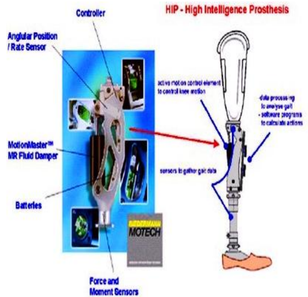
Fig. 5 – Prosthesis c with magnetic fluid damper
