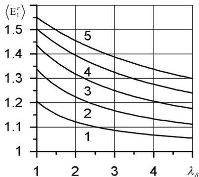
**Fig. 4** – Dependences of the relative macromodulus of the tetragonal structure nanocomposite (100 nm) as a function of the parameter  $\lambda_\delta = 2\delta\omega_1$ . The curves 1-5 are constructed for nanorods with diameter 10, 15, 20, 25 and 30 nm, respectively. The relative nanorod length is  $\lambda = 0.9$
