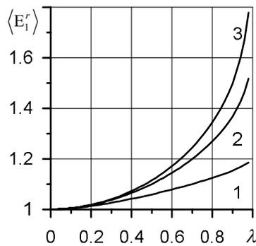
**Fig. 3** – Dependences of the relative macromodulus of the tetragonal structure nanocomposite (100 nm) as a function of the parameter  $\lambda$ , substrate thickness is  $\delta = 150$  nm, the curves 1-3 are plotted for nanorods with diameters 10, 20 and 30 nm, respectively
