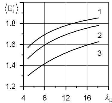
**Fig. 5** – Dependences of the relative macromodulus of the tetragonal structure nanocomposite (100 nm) as a function of the parameter  $\lambda_E = E_0/E$ . The curves 1-3 are plotted for different substrate thickness 100, 150, 300 nm, respectively. The relative nanorod length is  $\lambda = 0.96$
