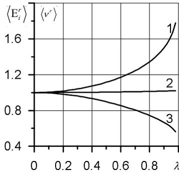
**Fig. 2** – Dependences of the relative macromoduli of the tetragonal structure nanocomposite ( $\omega_1 = 100$  nm) versus parameter  $\lambda$ . Substrate thickness is  $\delta = 150$  nm, nanotube diameter is 30 nm
