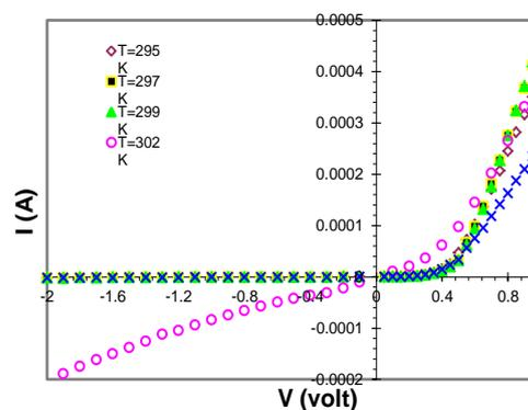
**Fig. 1** – I-V characteristics of Ga-Si(p) diode at different temperature around melting point of gallium
