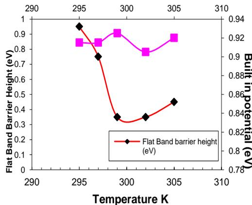
**Fig. 6** – Flat band barrier height and built-in volt potential variation with temperature for Ga-Si(p) diode
