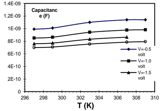
Fig. 4 – Capacitance vs Temperature of Ga-Si (p) Schottky diode at different voltages
