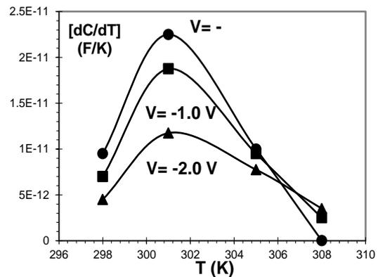
Fig. 5 –  $(dC) / (dT)$  (F / K) vs Temperature of Ga-Si(p) Schottky diode at different voltages
