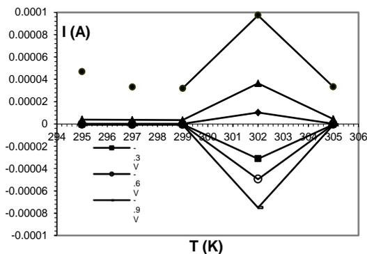
Fig. 3 – I-T Characteristics of Ga-Si(p) Schottky diode at different voltages after correction
