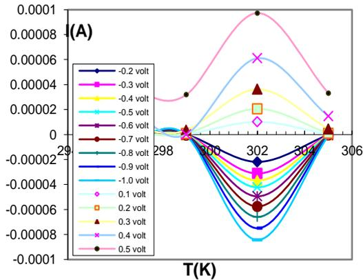
Fig. 2 – I-T Characteristics of Ga-Si(p) Schottky diode at different voltages before correction
