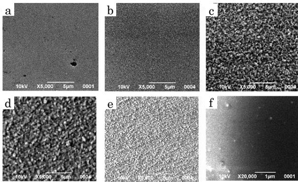
**Fig. 3** – Micrographs of ZnSe films obtained on glass substrates at the evaporator  $T_e = 800$  °C and substrate temperature  $T_s$ , °C: 100 (a), 200 (b), 300 (c), 250 (d), 350 (e), 500 (f)
