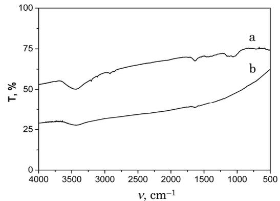
Fig. 2 – IR-spectra of ZnSe precursor after MW synthesis of elements (a) and after annealing in vacuum (b)
