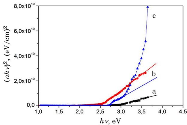
**Fig. 6** – Determination of the band gap optical width of ZnSe films obtained at different  $T_s$ , °C: 100 (a), 250 (b), 500 (c)
