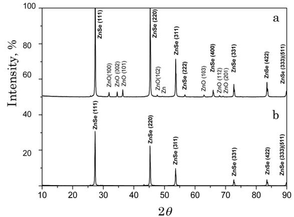
Fig. 1 – X-ray patterns of ZnSe precursor directly after MW synthesis of elements (a) and after annealing in vacuum (b)
