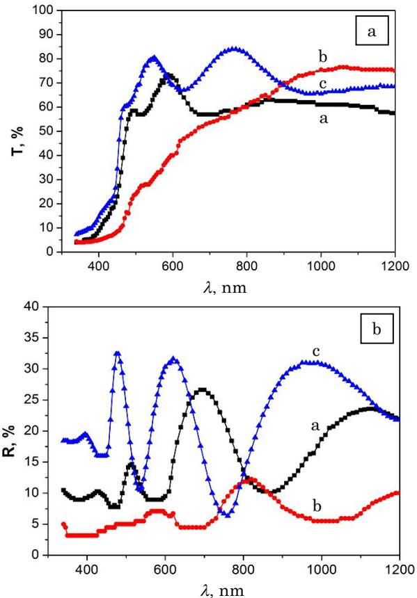
**Fig. 5** – Transmission (a) and reflection (b) spectra of ZnSe films obtained at different  $T_s$ , °C: 100 (a), 250 (b), 500 (c)
