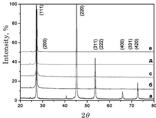
**Fig. 4** – X-ray diffraction patterns of ZnSe films obtained at different substrate temperatures  $T_s$ , °C: 100 (a), 200 (b), 300 (c), 250 (d), 350 (e), 500 (f)
