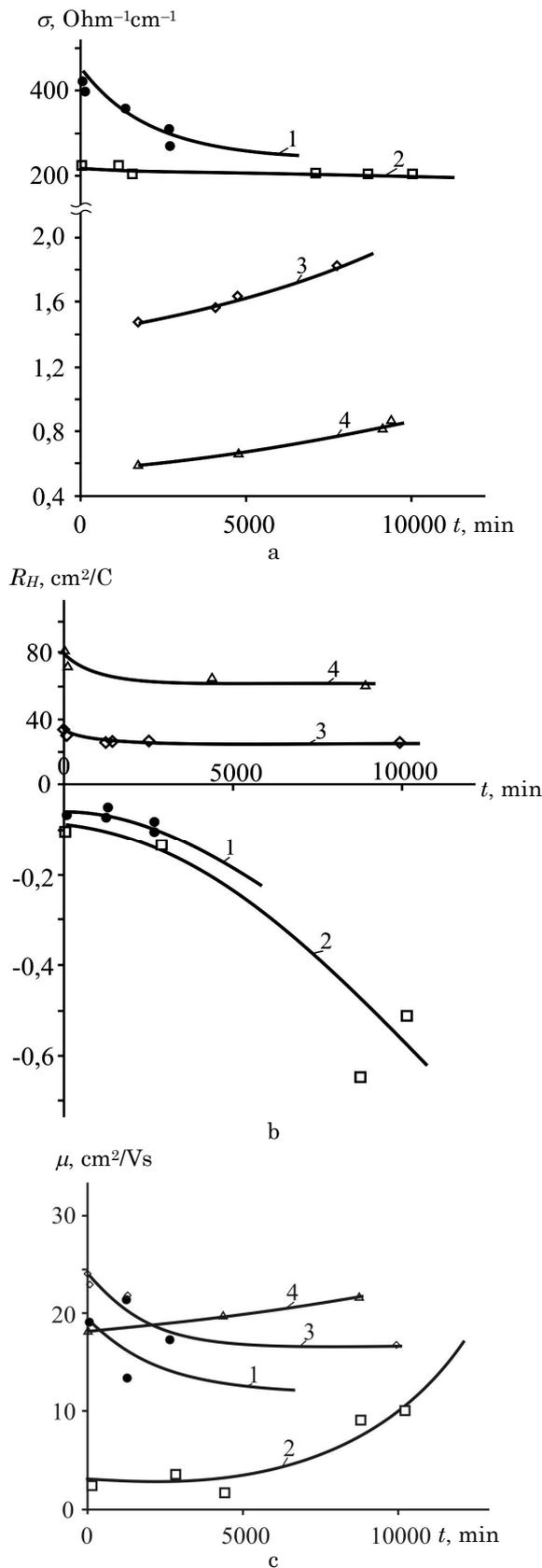
**Fig. 2** – Dependences of the conductivity  $\sigma$  (a), Hall coefficient  $R_H$  (b), and charge carrier mobility  $\mu$  (c) on the exposure time on air for PbTe:Bi films of different thickness  $d$ ,  $\mu\text{m}$ :  $\bullet$  (1) – 0,08;  $\square$  (2) – 1,08, and PbTe films with thickness  $d$ ,  $\mu\text{m}$ :  $\diamond$  (3) – 0,08;  $\Delta$  (4) – 0,3
