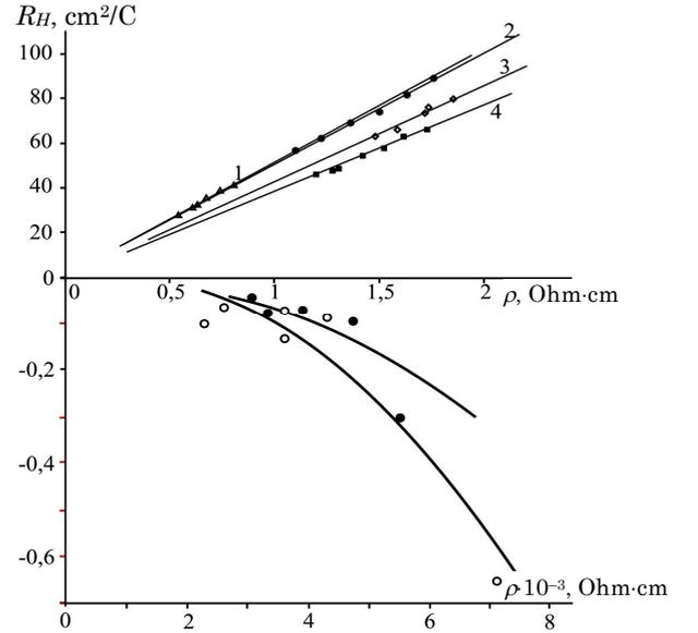
**Fig. 4** – Dependence of the Hall coefficient on the resistivity for PbTe films obtained on polyamide substrates (film thickness  $d$ ,  $\mu\text{m}$ : 1 – 0,08; 2 – 0,3; 3 – 0,54; 4 – 0,76), and for thin ( $d = 0,08 \mu\text{m}$ ) ( $\bullet$ ) and thick ( $d = 1,08 \mu\text{m}$ ) ( $\circ$ ) PbTe:Bi films on mica cleavages. Dots are the experiment; solid lines are the calculations by the formulas (1) and (2), respectively.
