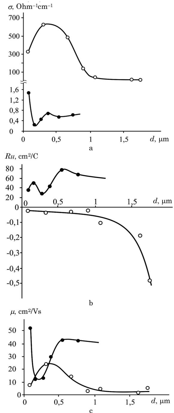
**Fig. 3** – Dependences of the conductivity (a), Hall coefficient (b), and charge carrier mobility (c) on the film thickness: PbTe ( $\bullet$ ) and PbTe:Bi ( $\circ$ ).
