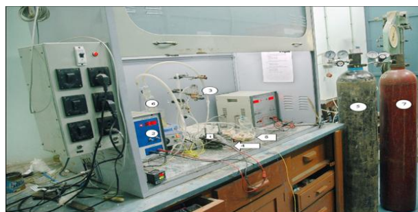
Fig. 1 – Experimental setup for performance study of PEMFC unit cell [Specifications: 1) PEMFC unit cell; 2) Constant current source; 3) Flow meters; 4) Probes connected to cell; 5) H 2 cylinder; 6) Humidifier; 7) O 2 cylinder; 8) Absorbers.
