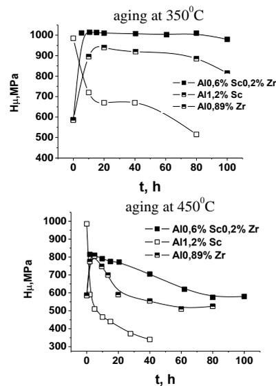
**Fig. 7** – Microhardness change after isothermal aging
