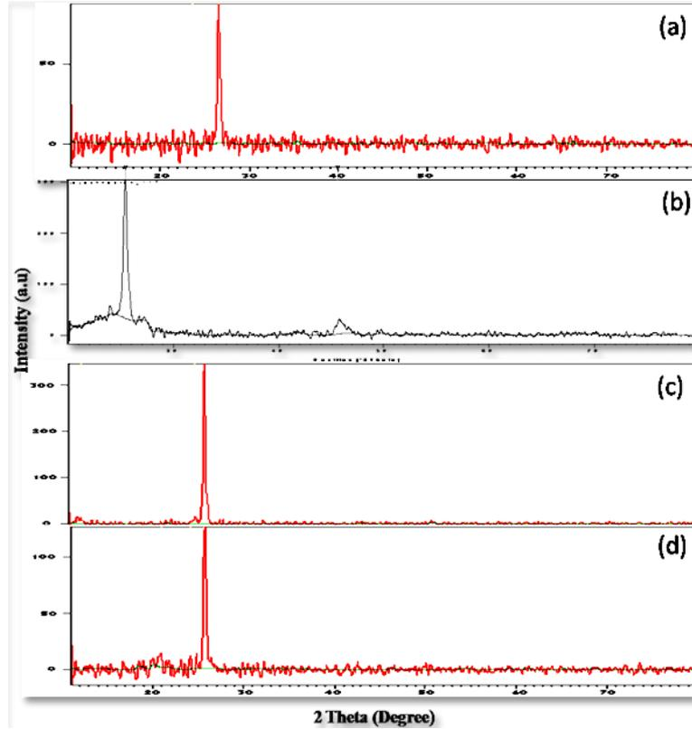
**Fig. 1** – XRD spectrum obtained for  $\text{Cd}_{1-x}\text{Zn}_x\text{Se}$  films with different  $x$  content
